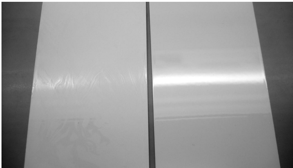
Figure 3.6: Picture of two standard plates with different surface status, to the left SebumTEFO, to the right AR. Note the difference in light reflection.
