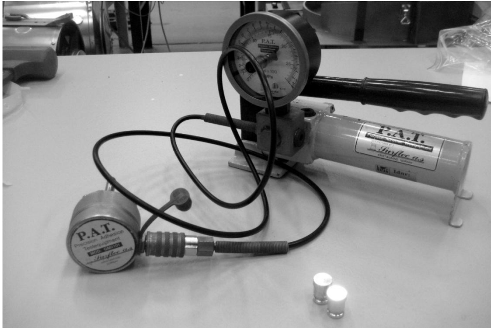
Figure 3.4: Picture of the pull-off adhesion test equipment, including two test elements.
