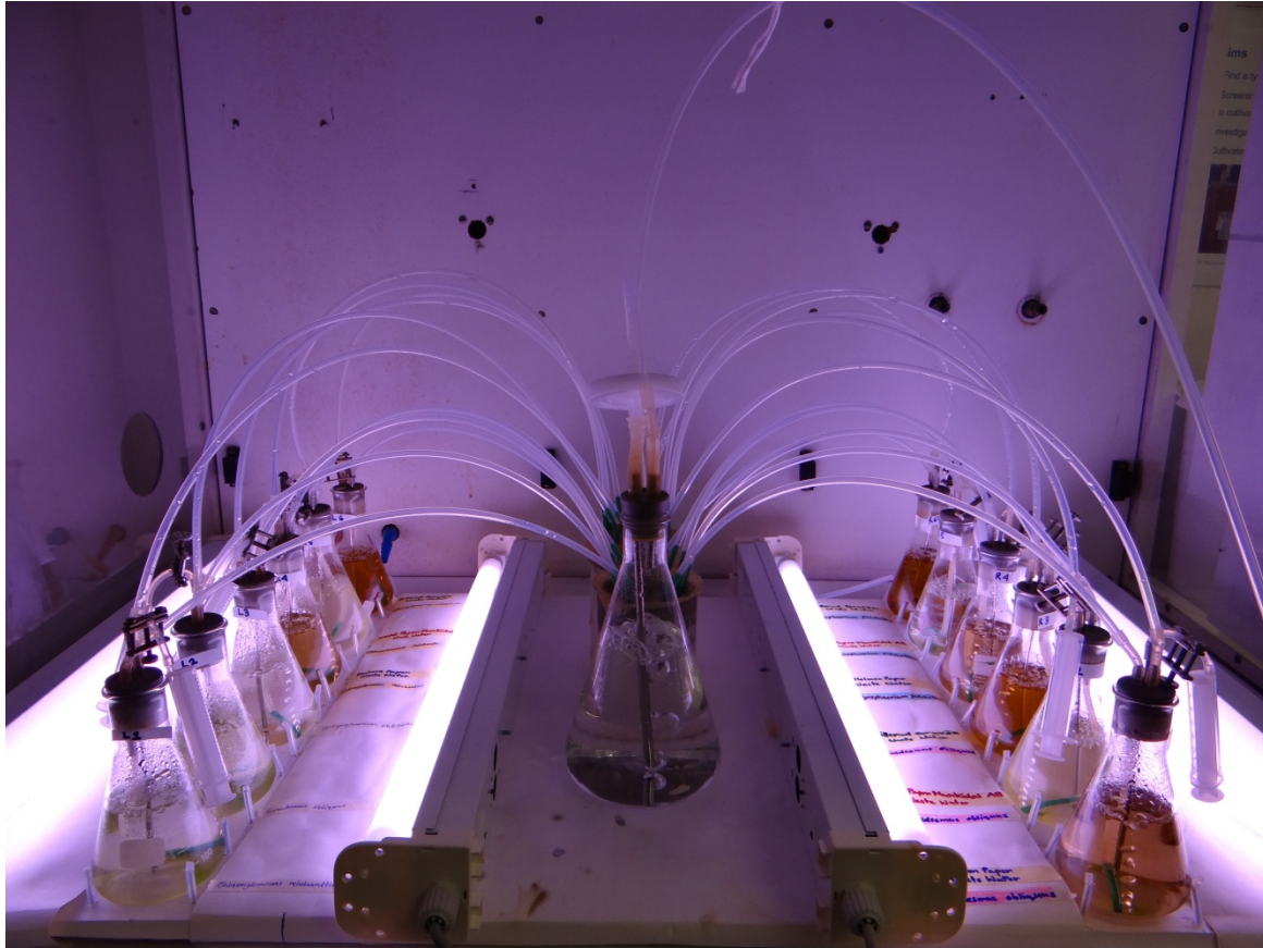
Figure 6: Gas distribution system used for screening. Picture taken during screening 1.
