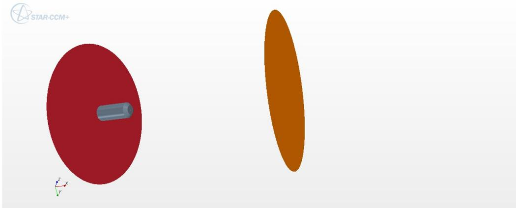
**Figure 3.1:** The geometry in the simulations, excluding the wall enclosing the system for clarity. The AdBlue injection orifice is 1mm in diameter and the surrounding annulus air injection orifice has an inner diameter of 1.6mm and an outer diameter of 1.9mm. The boundary to the left of the spray is a low velocity inlet. The inlet velocity is chosen to be 0.5 m/s to not affect the solution. The boundary to the right is a pressure outlet with no back pressure.
