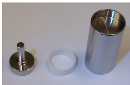
Figure 3.3: The electrodes in a Swagelok cell, left to right is top to bottom.
