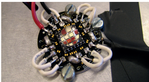
Figure 34. The heat sensor fastened onto the circuit board using cable tie and tape.
