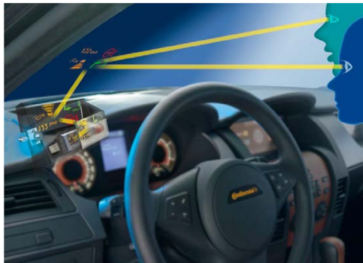
Figure 2.14 Schematic illustration of HUD (Telematic News, 2012)
