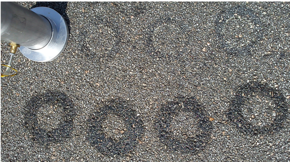
Figure A.15.: Photo of the test surface used for the in-situ measurement on a test patch. The eight circles is the in-situ sealant residue patches. The upper three patches seen in the photo is the residue from Plastilina, whereas the lower four are from Vaseline. In the upper left corner one can see the lower part of the impedance tube while performing a measurement.
