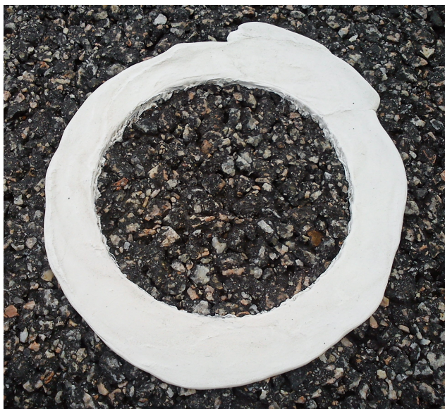
Figure A.23.: Photo of the ISO 10844:1994 specified test track surface layer. The inner diameter of the sealant circle is 80 mm. This photo shows the Tack-It sealant between the in-situ fixture and the surface layer. This sealant will be removed completely resulting in no residual debris, as seen for other sealants in Figure A.15.
