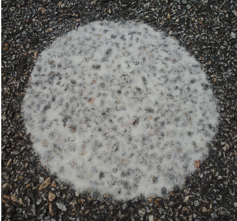
Figure 5.4.: Photo of performing the sand patch method. When this photo was taken, it just recently started to rain, hence the spots on the bright sand bed.
