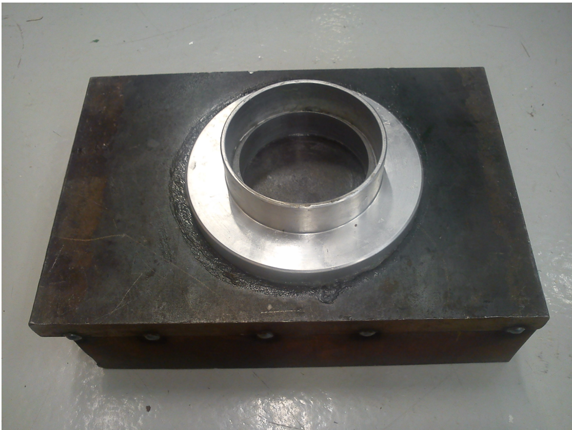
Figure A.1.: Photo of the in-situ test fixture attached to a thick steel plate used to perform an empty tube measurement.
