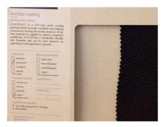
Slippery resisting coating which can be applied to almost any other type of material. Vital for preventing slip related injuries in hospital environment
