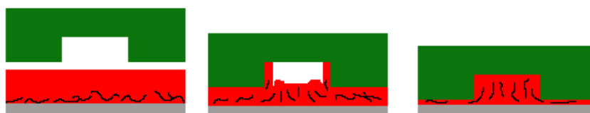
Figure 2.5: Expected nanotubes alignment due to NIL. Grey : Si substrate, black : nanotubes, red : polymer, green : mold. From left to right: The mold is placed upon the softened film. Then pressure is applied, leading to filling of the cavity as shown in figure 2.4 and displacing the nanotubes. Finally the film is dried, leaving the nanotubes aligned in the polymer film.
