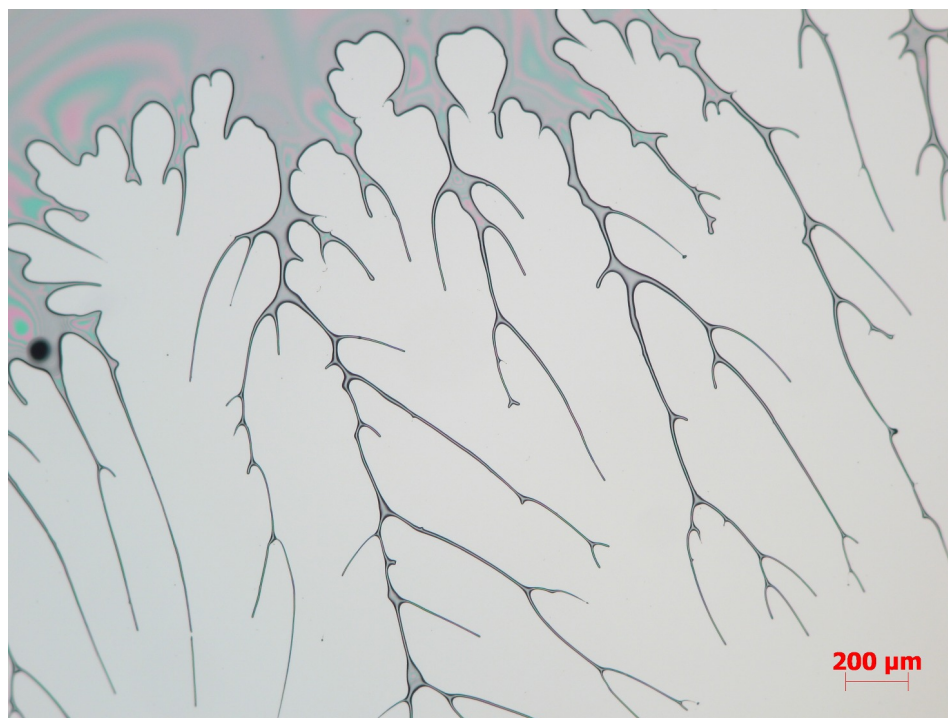
Figure 5.1: “Thin film” resulting from 10 wt % PS in o-DCB spun coated on a silicon substrate at 500 rpm
