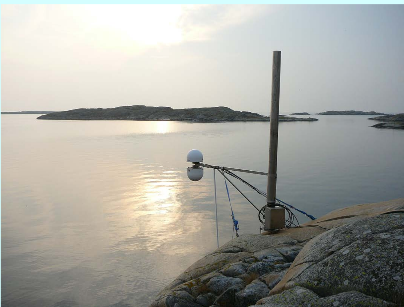
GNSS-R installation at the Onsala Space Observatory, for monitoring of the sea level.
