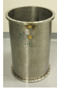
Fig. 2. Photograph of the finite circular cylinder cavity with its two loop-probes.
