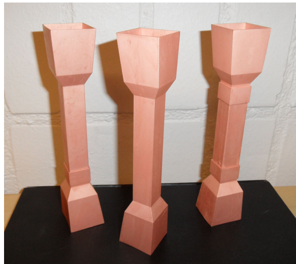
Fig. 3. 3D-printed plated waveguide parts.
