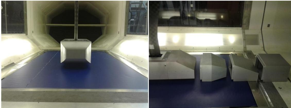
**Figure 17 Front and side view of the bluff-body models in Chalmers L2 Wind tunnel.**
