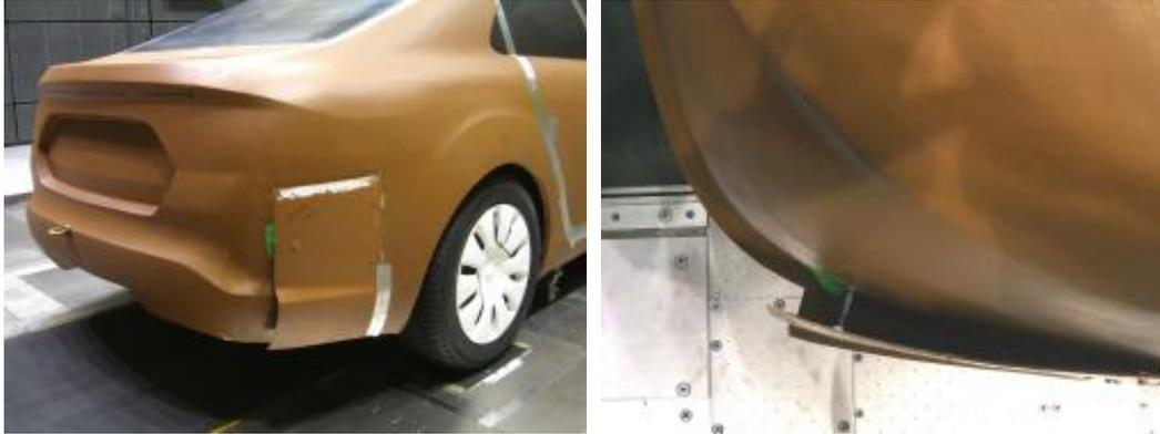
**Figure 43** Experiment carried out on a full size car at FKFS wind tunnel, by Saab Automobile.
