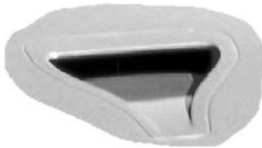
**Figure 14** Illustration of submerged NACA inlet duct.
