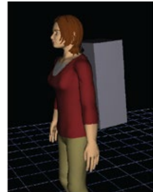
Fig.52 Tachymeter-dummy modelled in Catia V5. Testing of dimensions in ergonomic evaluation software Jack 7.1.
