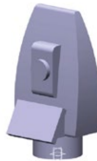
Fig.52 Tachymeter-dummy modelled in Catia V5. Testing of dimensions in ergonomic evaluation software Jack 7.1.
