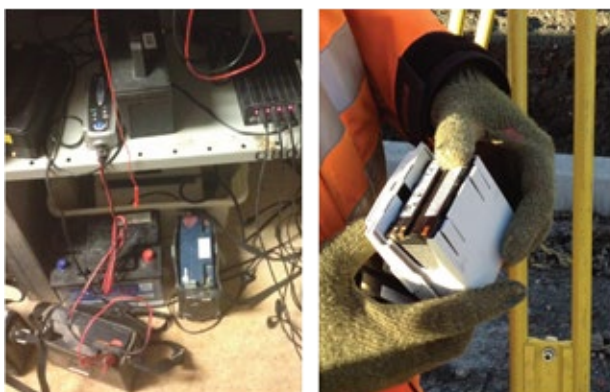
Fig.32 Large motorcycle batteries (6,4kg) used by Byggmätarna and a small battery pack (~0,2kg) used by Skanska.
