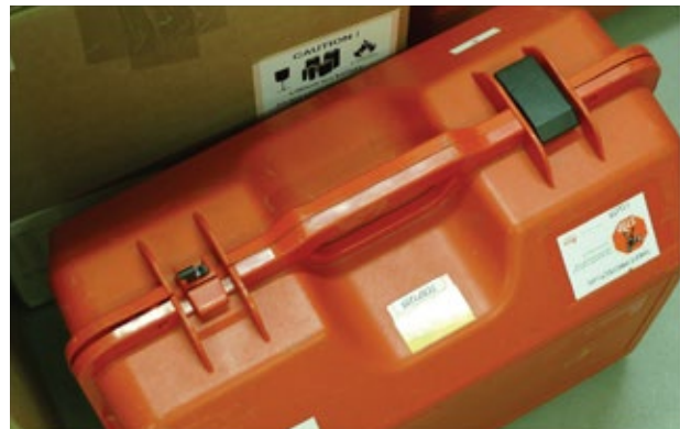
Fig.34 Broken latch on a protective case from Leica.
