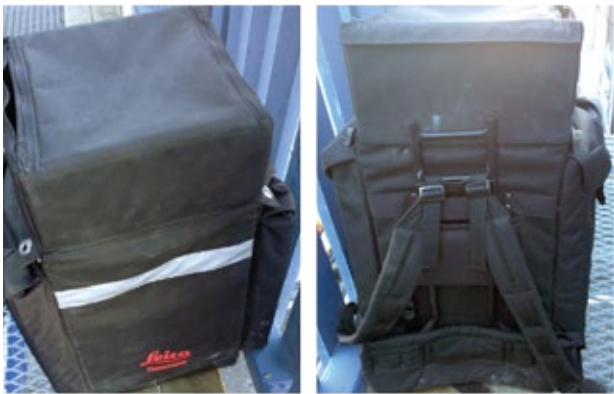
Fig.30 A soft backpack with an external frame. Used for transport and storage of tachymeters at Skanska and Lantmäteriet.
