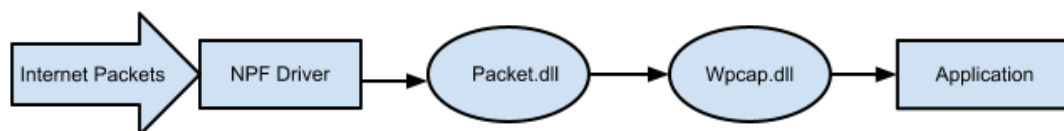
Figure 2.12: Schematic picture of how Winpcap work
