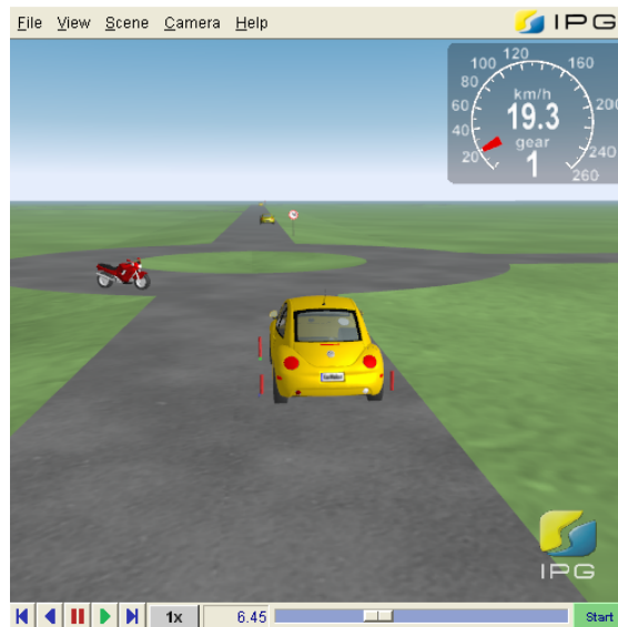
Figure 3.3.7: A GUI component, IPGMovie , visualizes the scenario simulation. It is possible to rewind and replay the simulation, which can be useful for debugging the control system's behaviour. IPGMovie also allows the user to record videos of the simulation post runtime.
