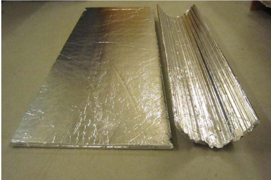
Figure 1.8 Two vacuum panels, to the left is a flat vacuum panel fitting as wall insulation and to the right is a curved insulation panel for use around pipes or columns. (Photo: Axel Berge)
