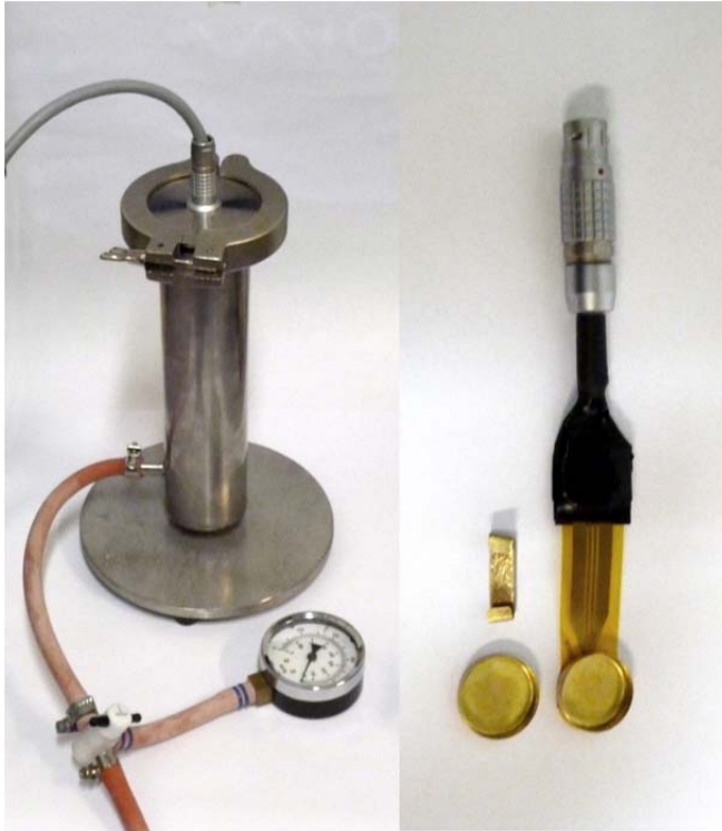
Figure 3.3 The equipment used for heat capacity measurements. To the right is the sensor, glued to a golden sample container and to the left is the steel tube, which can be evacuated, into which the sensor and the sample is inserted. (Photo: Axel Berge)
