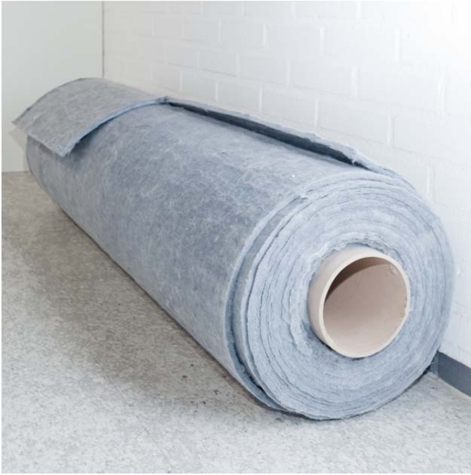
Figure 1.7 A roll of aerogel blanket. (Photo: Nina Zanders)
