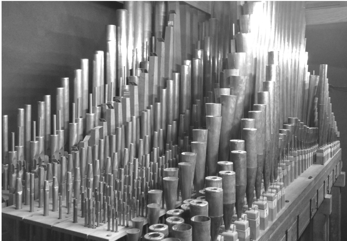
Figure 2.1 An example of symmetrical pipe placement on a windchest. Bass notes are placed in the middle and higher pitches on the sides. Different pipes in one line towards the wall on the left side are different ranks of the same note (Photo by Erkin Asutay).
