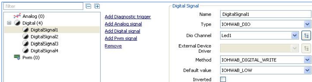
Figure 15: IO Hardware Abstraction configuration of LED1
