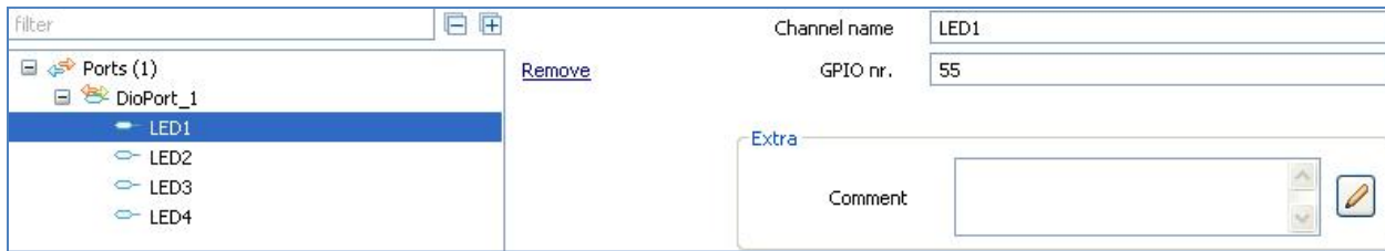
Figure 14: Dio configuration in BSW Builder
