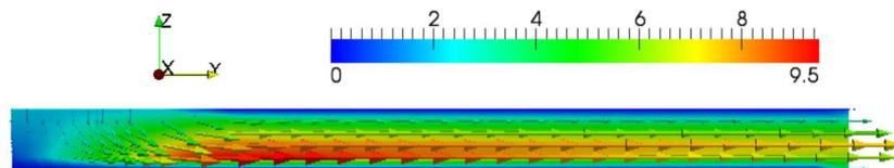
Figure 3.8: Velocity [m/s] in the cross section  $x = 50 \text{ mm}$  of the shielding plate, case 4. The left hand side is at the symmetry plane. The right hand side is at the edge of the shielding plate.
