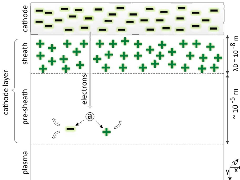
Figure 2.6: Scheme of sub-regions of an arc discharge
