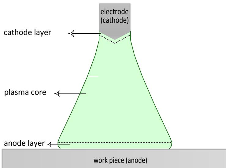
Figure 1.3: Schematic sketch of sub-regions in GTAW
