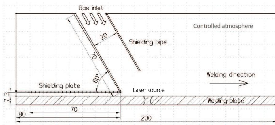
Figure 3.4: Partial cross section of the model [mm]
