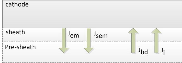
Figure 5.1: Current densities at the cathode layer
