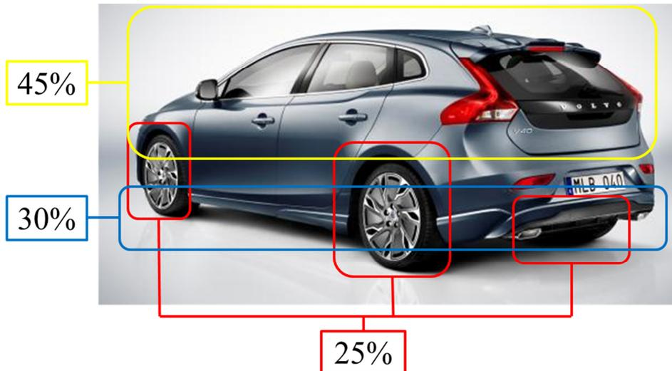
**Figure 3. Contributions to the aerodynamic drag from different parts of a passenger car**
