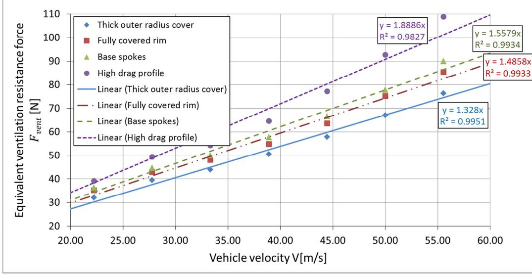
Figure 22. Equivalent ventilation resistance force vs vehicle velocity
