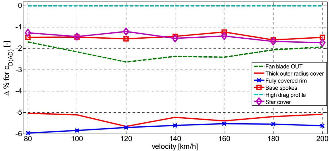
Figure 20. Aerodynamic resistance comparison for different rim configurations
