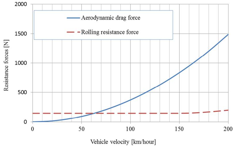
**Figure 4. Aerodynamic drag force and rolling resistance force versus vehicle velocity for a typical passenger vehicle**
