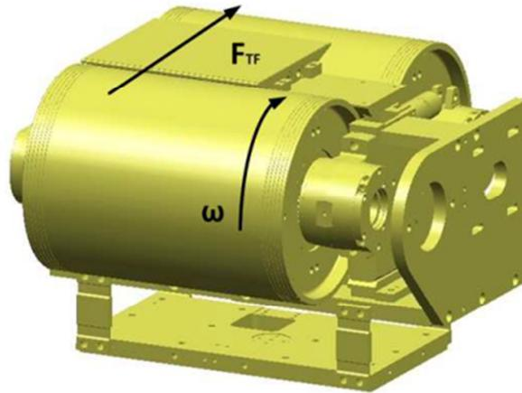
**Figure 14. Wheel drive unit (courtesy of Volvo Car Corporation)**
