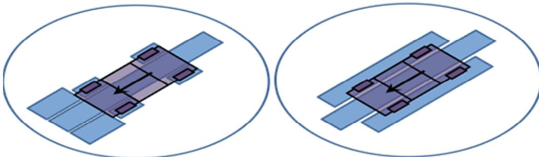
**Figure 10. T-belt and three-belt moving ground systems**
