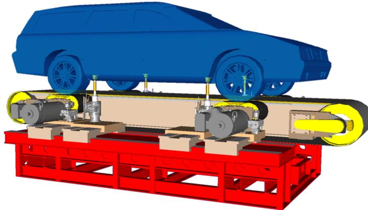
**Figure 9. Five-belt moving ground system used in Volvo aerodynamic wind tunnel (courtesy of Volvo Car Corporation)**
