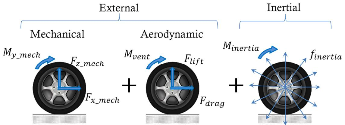
Figure 11. Forces acting on a rotating wheel
