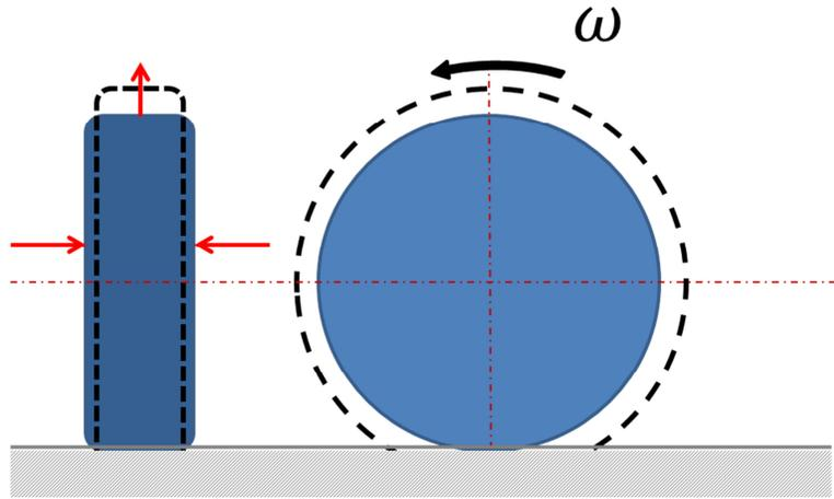
Figure 12. Deformations due to inertial forces
