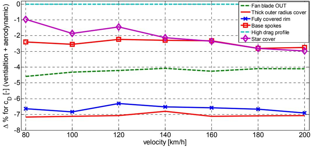
Figure 21. Total aerodynamic resistance comparison for different rim configurations
