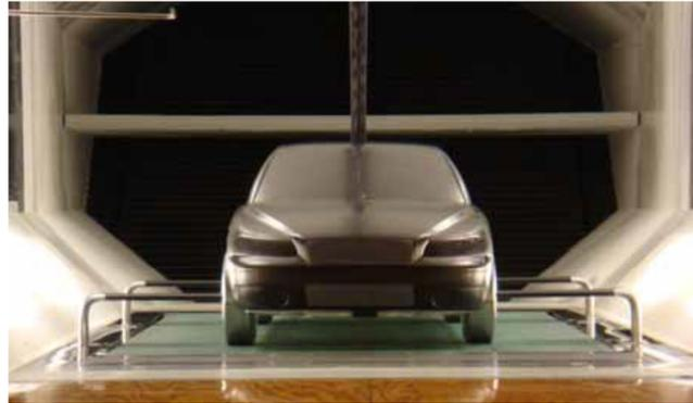
**Figure 7. Single belt moving ground set-up in Chalmers wind tunnel**
