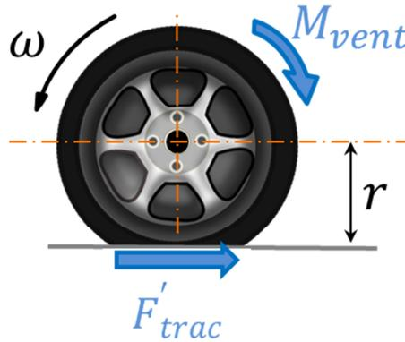
**Figure 18. Ventilation resistance measurement**
