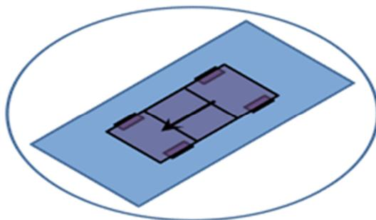
Figure 6. Single belt moving ground system
