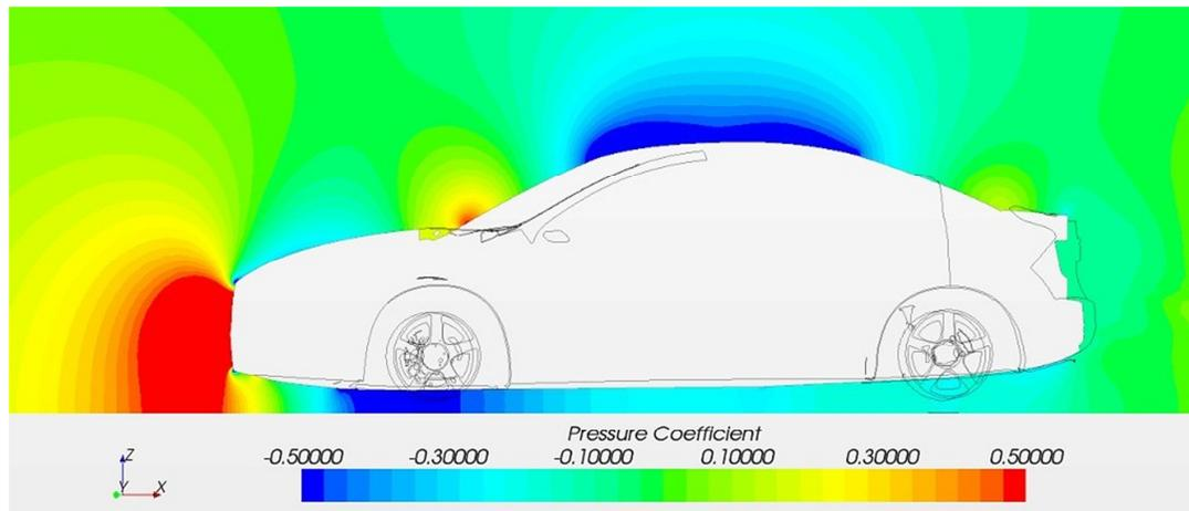
**Figure 5. Pressure coefficient at the symmetry plane of the vehicle**
