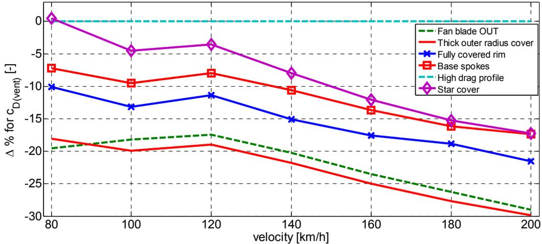
Figure 19. Ventilation resistance comparison for different rim configurations
