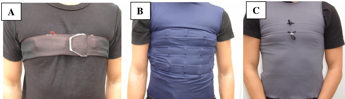
Figure 16. Examples of some tactile display concepts from FOI. These were developed in cooperation with the Swedish School of Textiles (University College of Borås). (A) FOI tactile torso belt as worn in the combat vehicle studies. (B) Tactile vest prototype with tactors. (C) A tactile vest prototype with adjustable size (Carlander, 2006).
