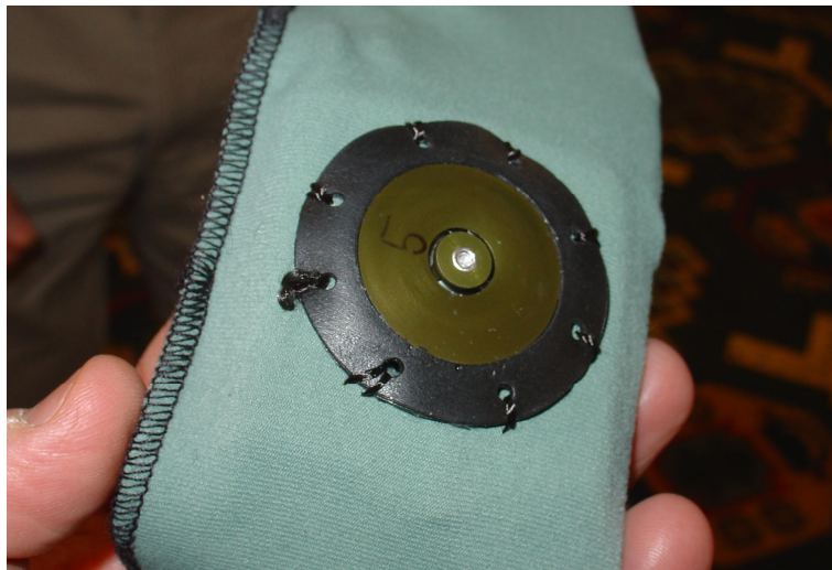
Figure 17. A linear actuator attached to a waist belt for conveying hand- and arm signals. The smaller circle centred on the tactor is the moving part. The picture is taken on a demo session at a North Atlantic Treaty Organisation (NATO) Research and Technology Organisation (RTO) HFM-122 group meeting in Breckenridge, Colorado, USA, 2006.
