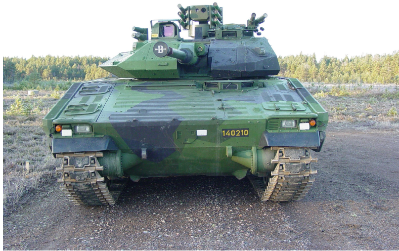
Figure 24. The Combat Vehicle 90 (CV 90) technology demonstrator as used in the WCS experiment (Picture credit to Jan Fredriksson, MSS Skövde, 2005).
