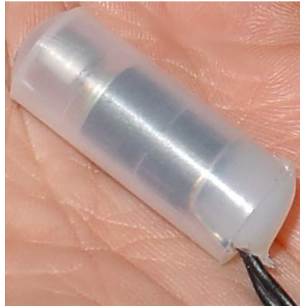
Figure 15. A tactor developed by the Swedish Defence Research Agency, FOI. It is based on a rotary DC motor encapsulated in a PVC cylinder.
