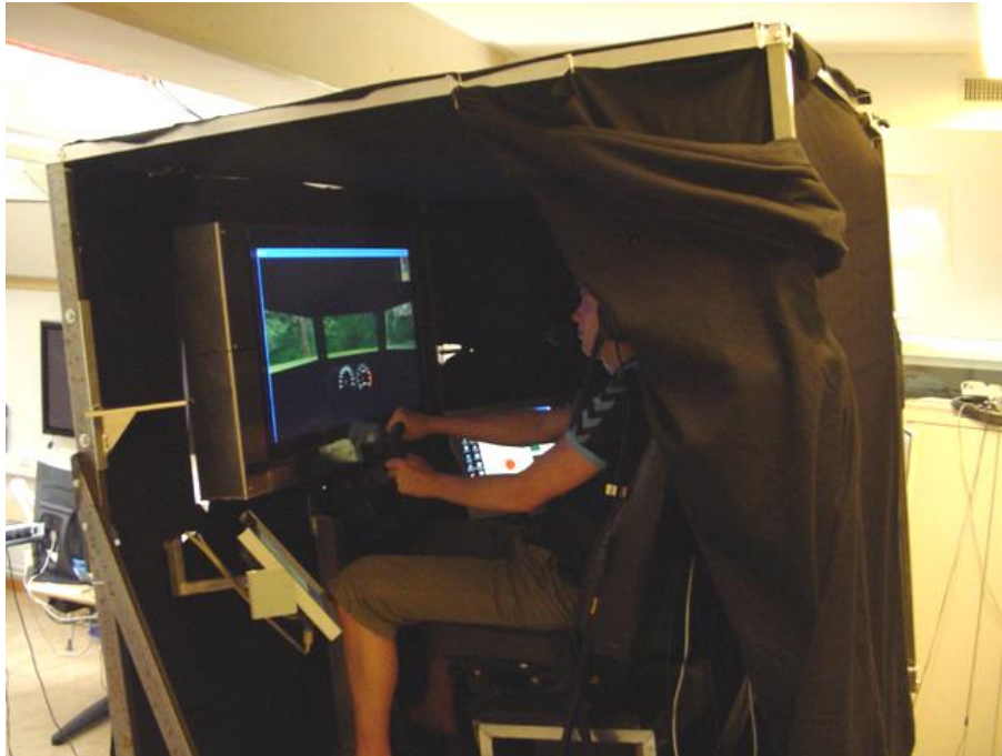
Figure 29. The FOI “CV90 simulator” based on a motion platform with 6 degrees of freedom. Screens for presenting the HDD information and handling radio calls are seen on the lower left and right of the participant. Vehicle information and out-the-window view is displayed on the large screen in front of the participant.
