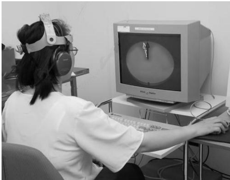
Figure 6. A 3D audio system with a head tracker, headphones and a corresponding visual interface. The head tracker, attached to the head of the participant compensate for head movements allowing a more natural sound localization process (Chen & Carlander, 2003b).
