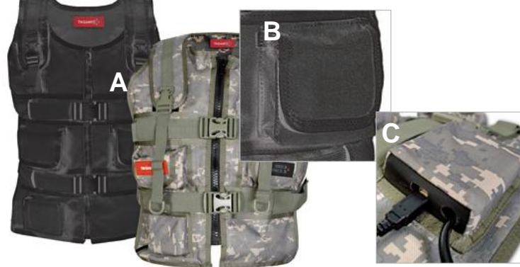
Figure 20. A) Two versions of 3rd Space FPS tactile gaming vest. B) The Pneumatic tactors are embedded in small pouches around the vest. C) The vest connects via a control box over USB (Coxworth, 2010).
