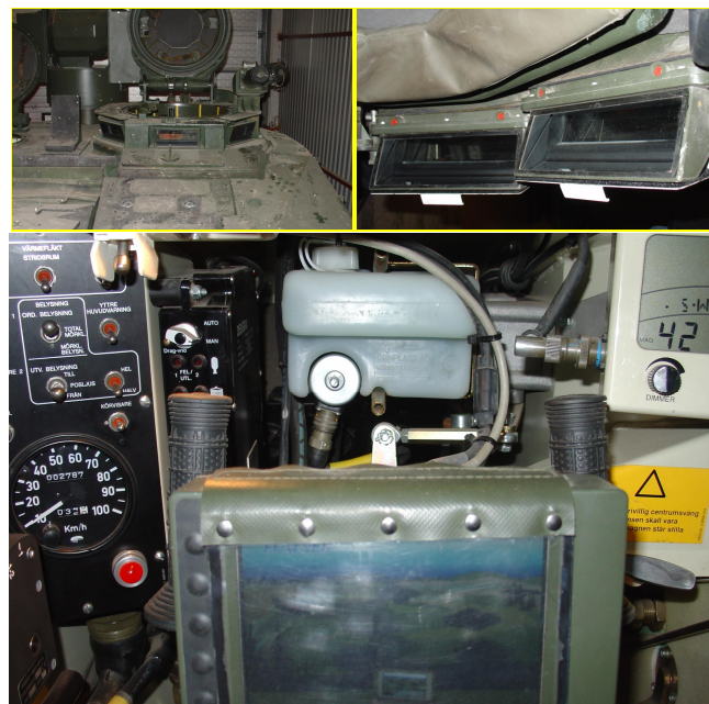
Figure 1. Pictures showing elements of the working environment for the CV90 1 driver. Top left, the prismatic that the driver use for outside view, top right, inside view of the prismatic. Bottom, steering handle with 2D visual information. Navigational equipment (far right) and engine controls (far left) are also seen.
