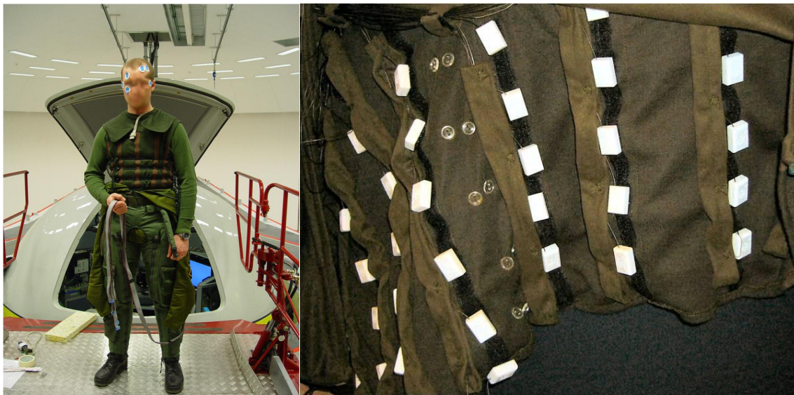
Figure 21. To the left, a pilot prior to the experiment. The pilot is equipped with the necessary flight equipment, tactile vest and electrodes for physiological measurements. To the right, the inside of the TNO tactile vest showing the factors as housed in small white cubes.
