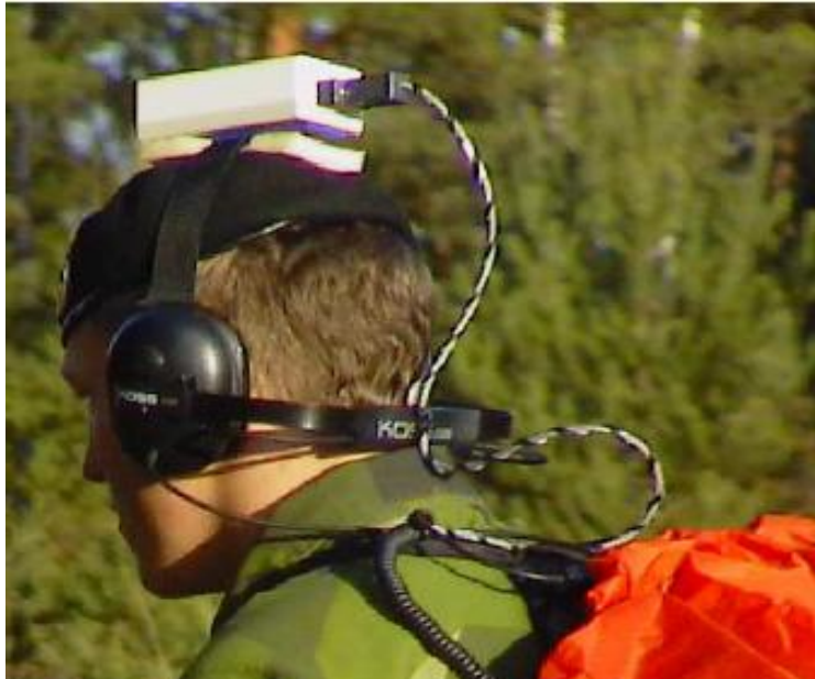
Figure 11. 3D audio system as used by Eriksson et al. (2008, p. 1283). A dismounted soldier is equipped with headphones and a digital compass (the white box on top of the head). Picture is used with permission from SAGE ( http://pro.sagepub.com/content/52/18/1282 ).
