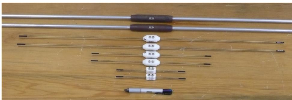
**Figure 3.6:** Dipoles of 60 MHz, 180 MHz, 400 MHz and 700 MHz
