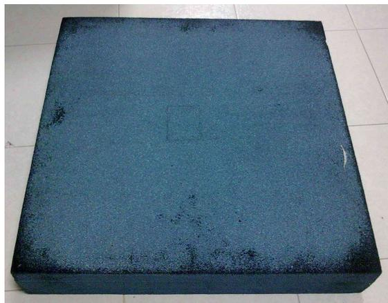
**Figure 3.5:** RF absorber material
