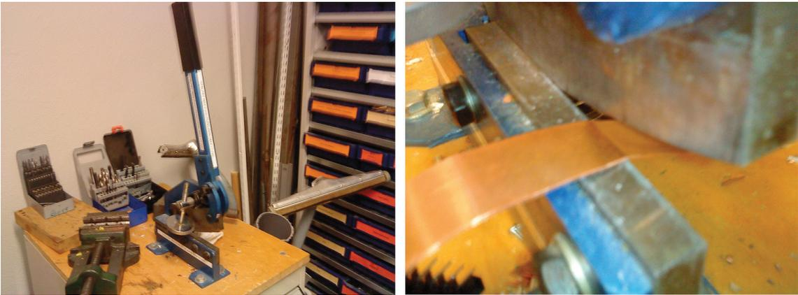
Fig. 3.10 Cutting the copper foil.
