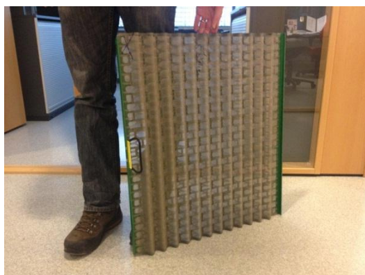
Figure 5.5. A small shaker screen with pyramid shaped mesh.
