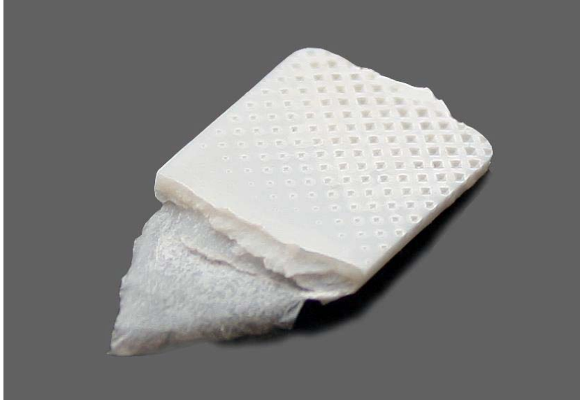
Figure 22: Skin formation on injection moulded TBV specimen.
