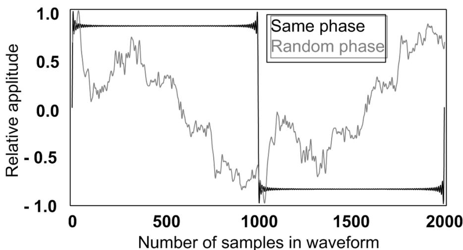
Figure 4.3: Example of two harmonics limited waveforms, both containing 100 odd harmonics and 2000 samples per period. The black waveform has all phase shifts equal to zero and the gray one has randomly distributed phase shifts.
