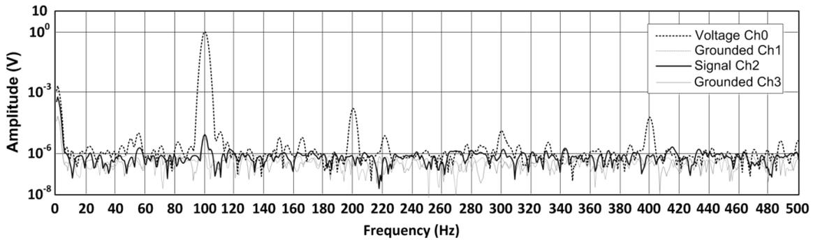
Figure 3.10: Noise levels of the DAQ card at low frequency, Ch0 is measuring a 7 V, 100 Hz sinusoidal voltage through a voltage divider, Ch1 and Ch3 are directly grounded and Ch2 is connected through an amplifier and a capacitive shunt to ground.
