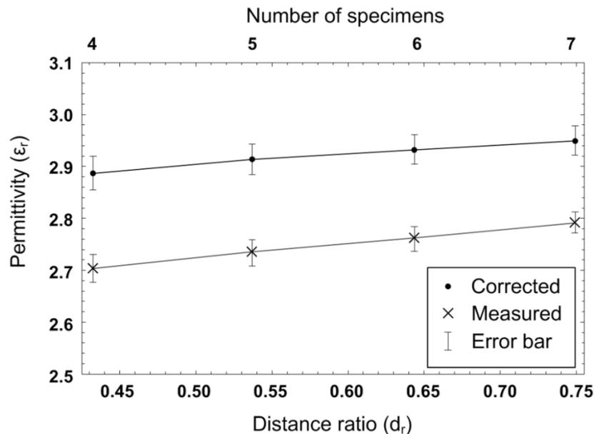
Figure 6.7: Measured and corrected permittivity of several layers of PET film specimens (about 0.1 mm each) in 1 mm fixed test gap, the applied voltage for all the measurements were 1 kHz and 7 V.
