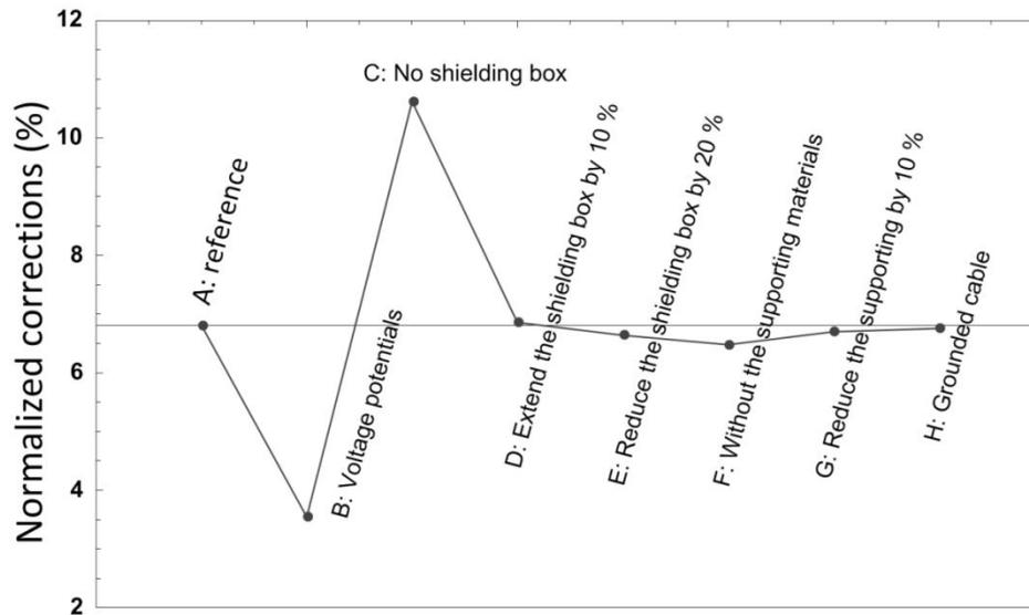
Figure 6.5: Normalized correction factor (%) for eight scenarios considered in the model.
