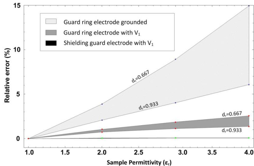
Figure 6.9: Relative error of the calculated “measured” permittivity that listed in table 6.1.
