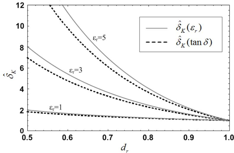
Figure 5.7: Noise sensitivity parameter,  $\hat{\delta}_K$ , as a function of the gap fill factor,  $d_r$ . The solid lines are valid for  $\epsilon_r$  and the dashed lines for  $\tan \delta$ , with  $\epsilon_r = 5, 3, 1$  from top of the figure. In the figure, a loss factor level of 10% is used to make the difference visible. Already at 1% the curves for  $\epsilon_r$  and  $\tan \delta$  are almost identical.
