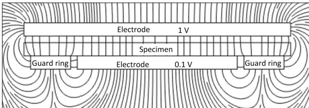
Figure.6.1: Electric field distribution of two parallel disk electrodes with guard ring, the ring electrode is grounded.
