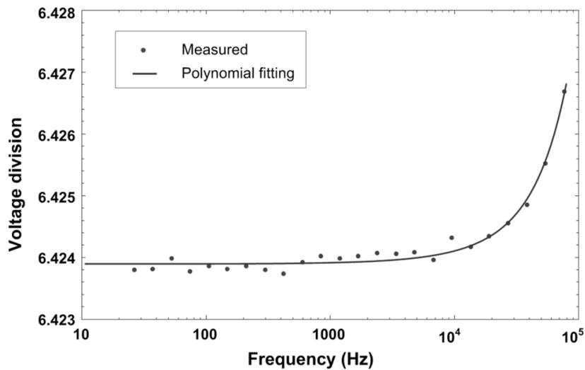
Figure 3.7: The measured and curve fitted absolute value of the voltage division.
