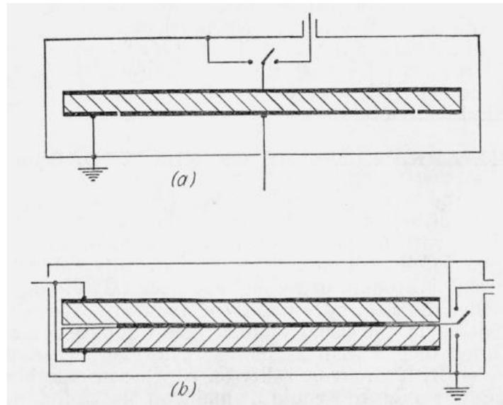
Figure 2.9: Two electrode arrangements to determine dielectric permittivity, suggested in paper [3].
