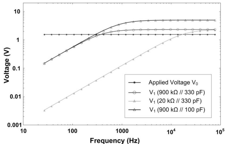
Figure 3.3 Swept voltages  $V_0$  (a 10 V sinusoidal waveform measured through a 6.4:1 voltage divider) and response voltages  $V_1$  over three different shunts (900 k $\Omega$  // 330 pF, 20 k $\Omega$  // 330 pF and 900 k $\Omega$  // 100 pF), test object capacitance  $C_{to} = 100$  pF.
