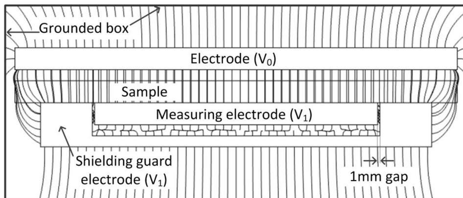
Figure.6.8: Electric field distribution of two parallel disk electrodes with shielding guard electrode. The voltage potentials generated at measuring electrode and the shielding guard electrode are expected to be the same.
