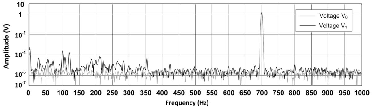
Figure 5.4: Measured frequency spectrum of applied voltage  $V_0$  (7 V and 700 Hz) and its responding voltage  $V_1$  from a polycarbonate specimen with charged surface in contact-free electrode arrangement.
