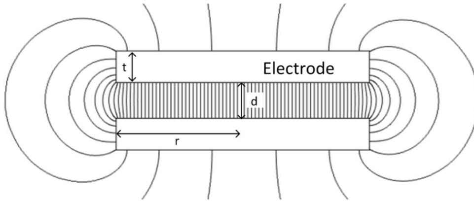
Figure 2.6: Electric field distributions between two parallel equal circular electrodes
