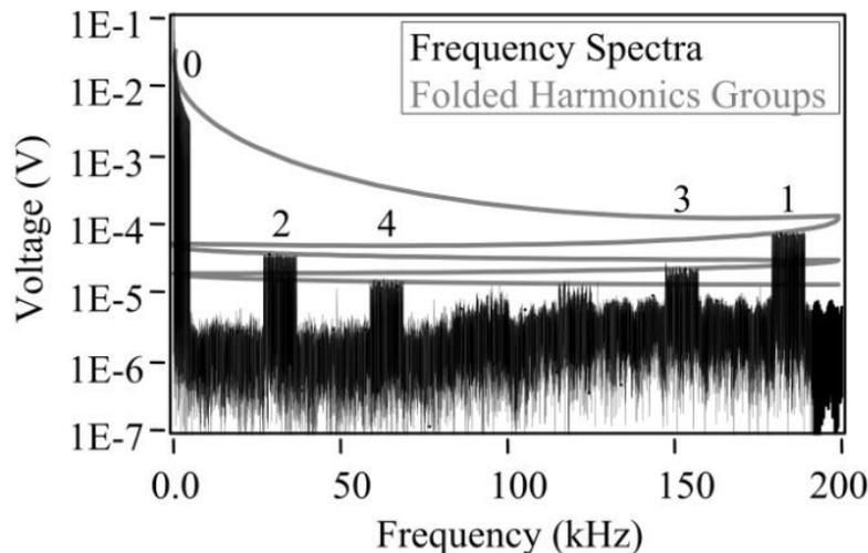
Figure 4.5: Frequency spectra of harmonics limited voltage waveform with folded harmonics groups (4320 samples in waveform,  $f_f = 50$  Hz, 50 odd harmonics); DAQ card sampling rate: 400 kS/s, waveform generation rate: 216 kS/s.
