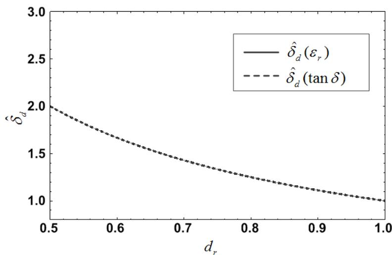
Figure 5.6: Normalised distance sensitivity parameter,  $\hat{\delta}_d$ , as a function of gap fill factor,  $d_r$ . The results for  $\varepsilon_r$  and  $\tan\delta$  are the same irrespective of the value of  $\varepsilon_r$ .
