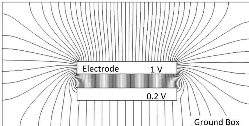
Figure 2.7: Electric field distributions of two parallel circular electrodes enclosed by a ground box; the electric potential of top electrode is 1 V and the bottom electrode is 0.2 V.
