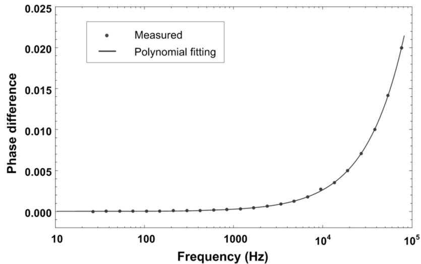
Figure 3.8: The phase difference between  $V_{in}$  and  $V_{out}$  of the voltage divider.
