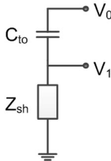
Figure 3.1: Principal circuit for dielectric response measurement of a test object ( $C_{to}$ ). The shunt impedance ( $Z_{sh}$ ) is used to measure the current passing through the test object.
