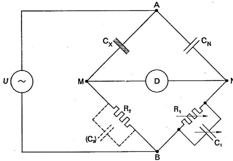
Figure 2.2: Circuit diagram of high voltage Schering bridge [1].
