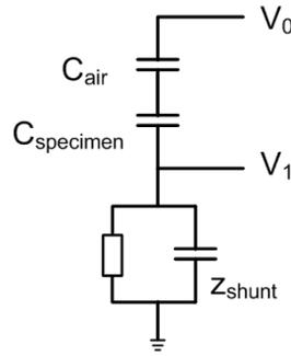
Figure 6.3: Circuit model for calculating generated voltage on the measuring electrode.
