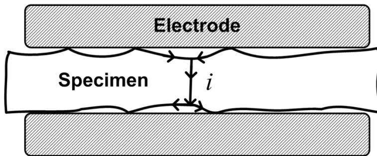
Figure 2.3: Surface current paths due to insufficient contact between specimen and electrodes.
