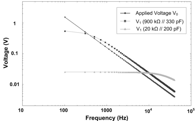
Figure 3.2 Applied voltage  $V_0$  (a square shape like voltage waveform contents 200 odd harmonics, it is measured through a 6.4:1 voltage divider) and response voltage  $V_1$  measured over two different shunts (900 k $\Omega$  // 330 pF and 20 k $\Omega$  // 200 pF), the test object has capacitance  $C_{to} = 100$  pF.
