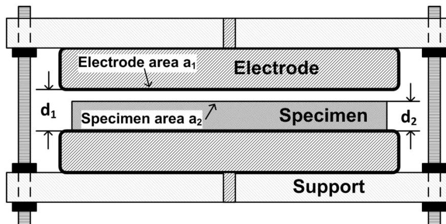
Figure 5.1: Sketch of the contact-free electrode arrangement,  $d_1$  is the distance between two parallel electrodes and  $d_2$  is the thickness of tested material,  $a_1$  is the area of electrode and  $a_2$  is the specimen area.
