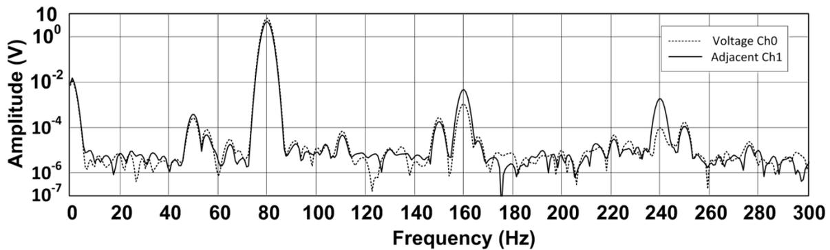
Figure 3.4: Applied voltage on Ch0 only (7 V and 80 Hz sinusoidal) and the corresponding crosstalk in the adjacent Ch1 which is connected through a capacitive shunt (a 330 pF capacitor in parallel with a 900 k $\Omega$  resistor) to ground. The sampling rate of DAQ card is set to 200 kS/s.
