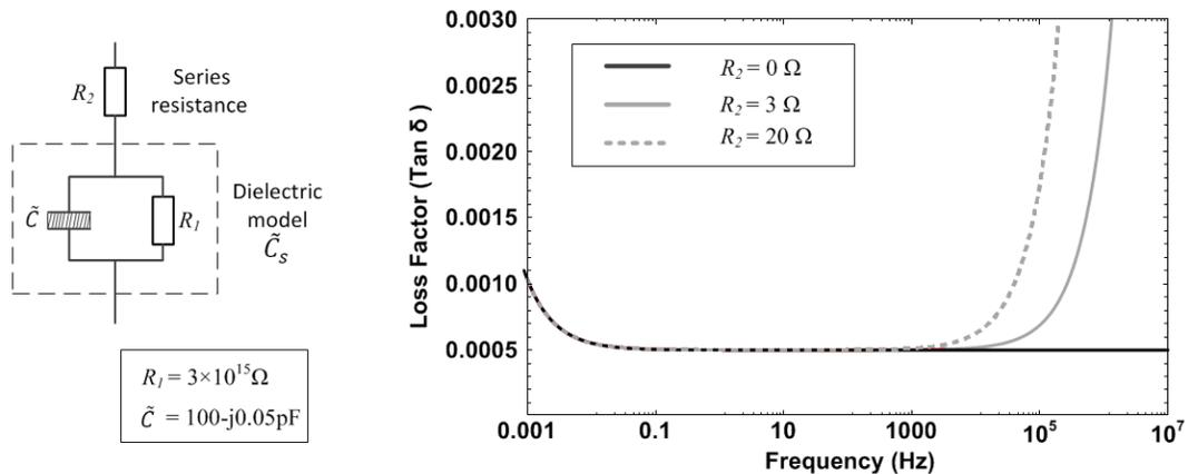
Figure 2.4: Model of dielectric with different series resistances and the resulting total losses.
