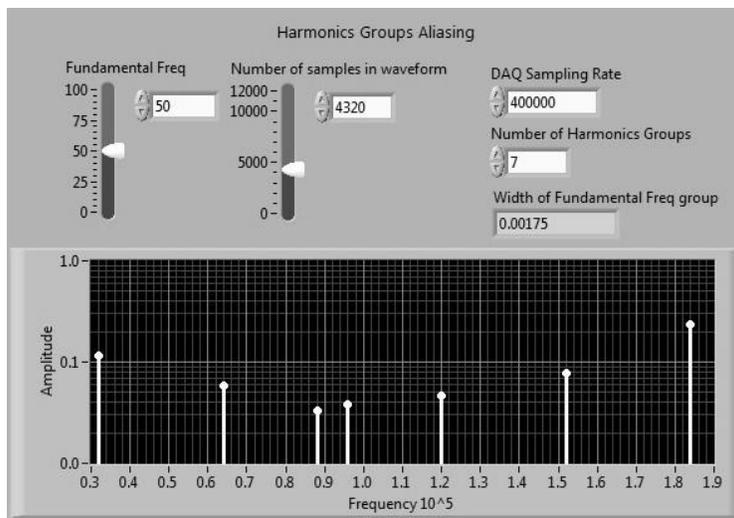
Figure 4.6: A support tool for predicting the position of folded-back harmonic groups with specified fundamental frequency, number of samples in the waveform and DAQ card sampling rate (the data from Figure 4.5 are analyzed).
