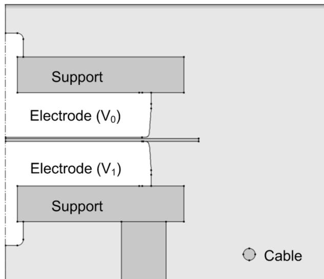
Figure 6.4: FEM model of electrode arrangement with a grounded cable nearby.
