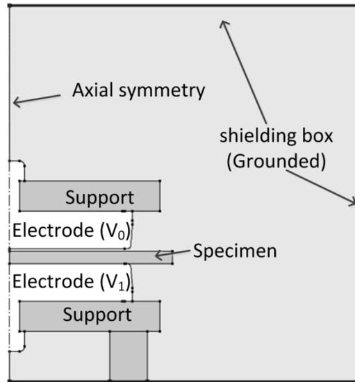
Figure 6.2: 2D symmetric finite element model for geometric influences correction in permittivity determination
