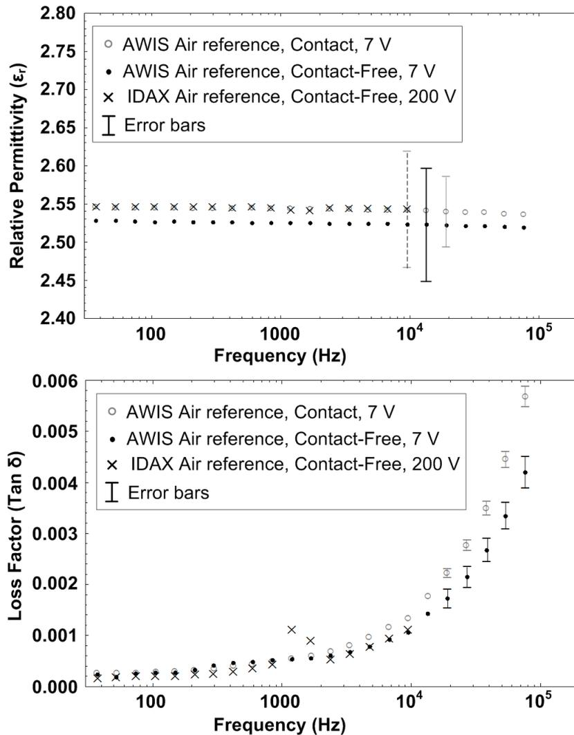
Figure 5.10: Relative permittivity and loss factor of a 0.75 mm thick polycarbonate specimen measured by AWIS with contact and contact-free electrode arrangement and measured by IDAX with contact-free electrode arrangement, similarly to figure 5.9. In the measurements the air reference method was applied.
