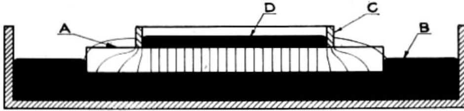
Figure 2.5: Mercury electrode arrangement suggested in [2].
