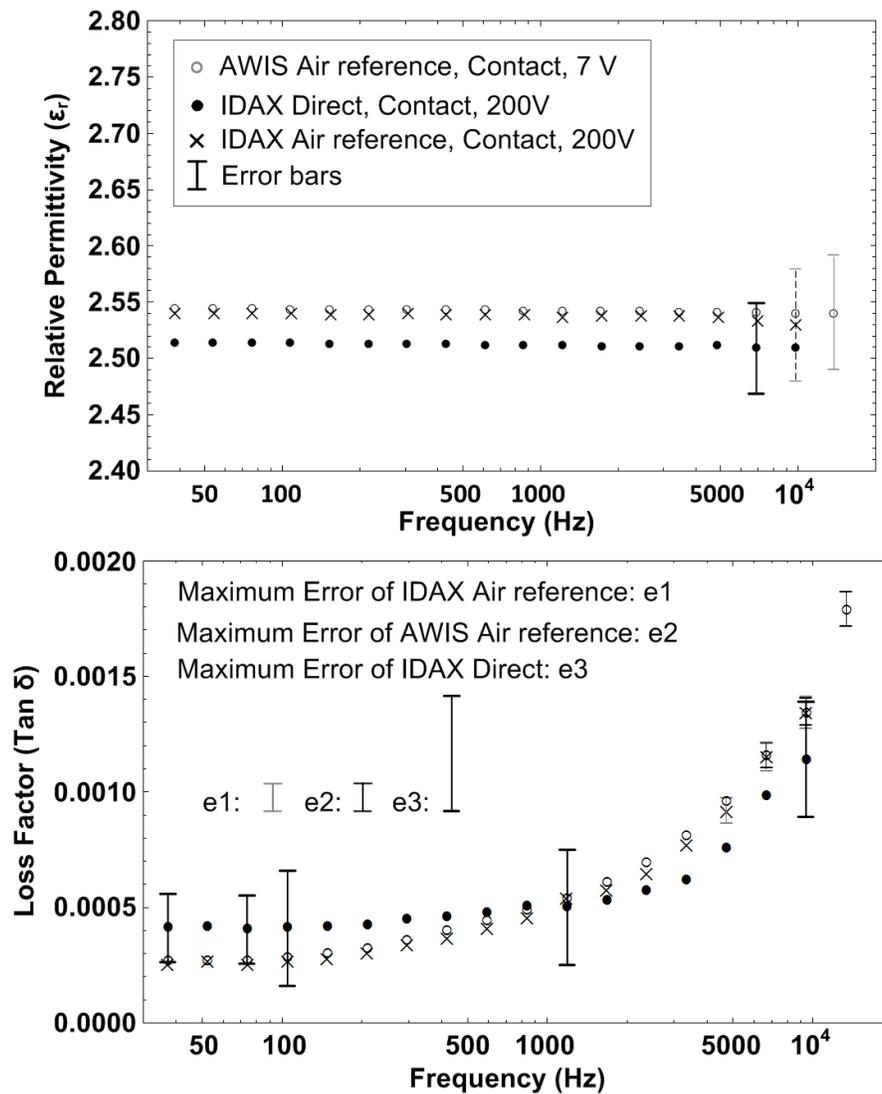
Figure 5.9: Relative permittivity and loss factor of 0.75 mm thick polycarbonate specimen measured by AWIS with the air reference method and measured by IDAX with both the air reference method and the direct method in the contact electrode arrangement. In order to improve the readability, only few data points are marked with error bars as they are in a same uncertainty range for each frequency.
