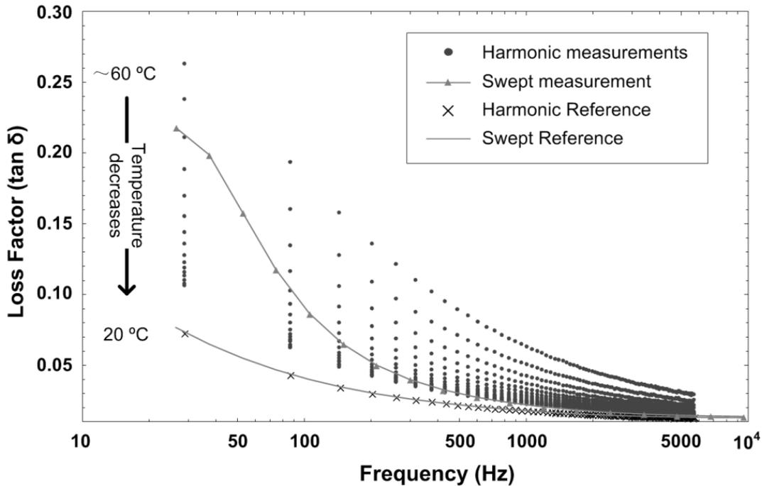
Figure 4.7: Frequency dependence of loss factor for dry pressboard sample measured under continuously changing temperature (from 60 °C down to 20 °C), the time interval between each swept frequencies point and between each harmonic measurement are the same, 5 seconds.
