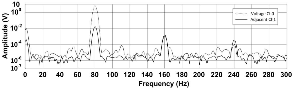
Figure 3.5: Applied voltage on Ch0 only (7 V and 80 Hz sinusoidal) and the corresponding crosstalk in an adjacent Ch1, which is connected through a voltage follower and in series with a capacitive shunt (a 330 pF capacitor in parallel with a 900 k $\Omega$  resistor) to ground. The sampling rate of DAQ card is set to 200 kS/s.
