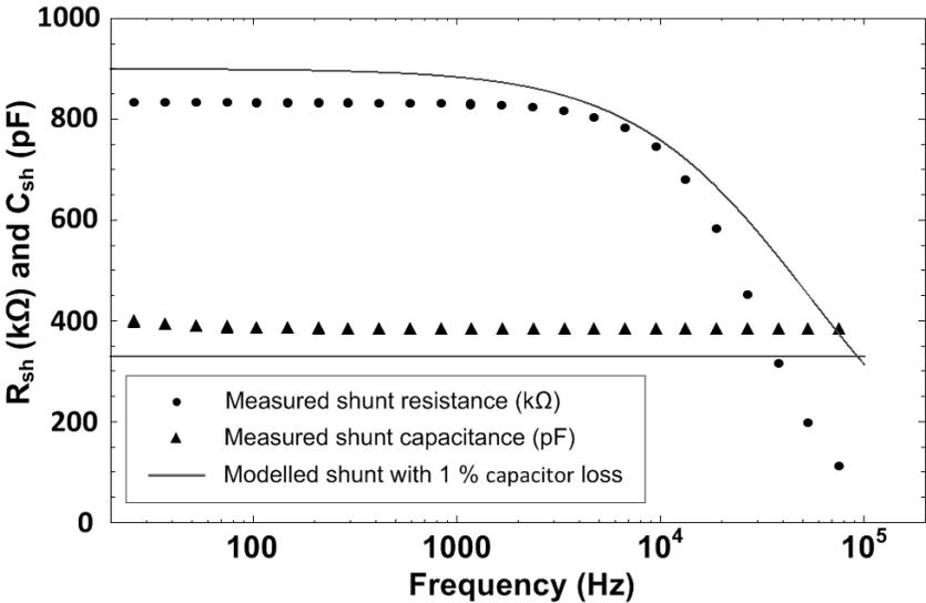
Figure 5.2: Measured and modeled shunt resistance and capacitance of the AWIS setup, modeled shunt circuit with nominal value of shunt components, including 1% shunt capacitor loss, is used.
