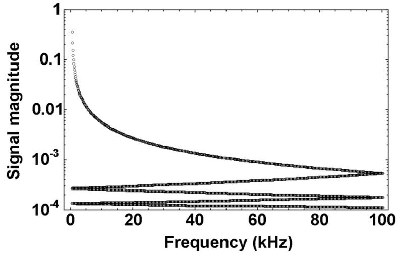
Figure 4.2: Folded harmonics of a square voltage waveform with fundamental frequency 42 Hz and a sampling rate of 200 kS/s. As the square wave has linearly decreasing harmonic amplitudes, the original frequency is here reflected in the signal magnitude.
