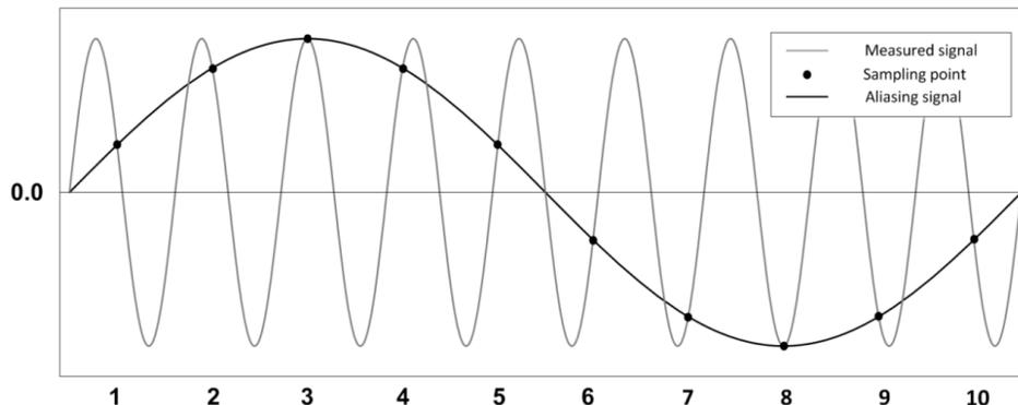
Figure 4.1: Example of aliasing in periodic sampling, a sinusoidal signal  $f = 0.9$  sampled with  $f_s = 1$  and its corresponding aliasing signal with  $f_a = 0.1$ .
