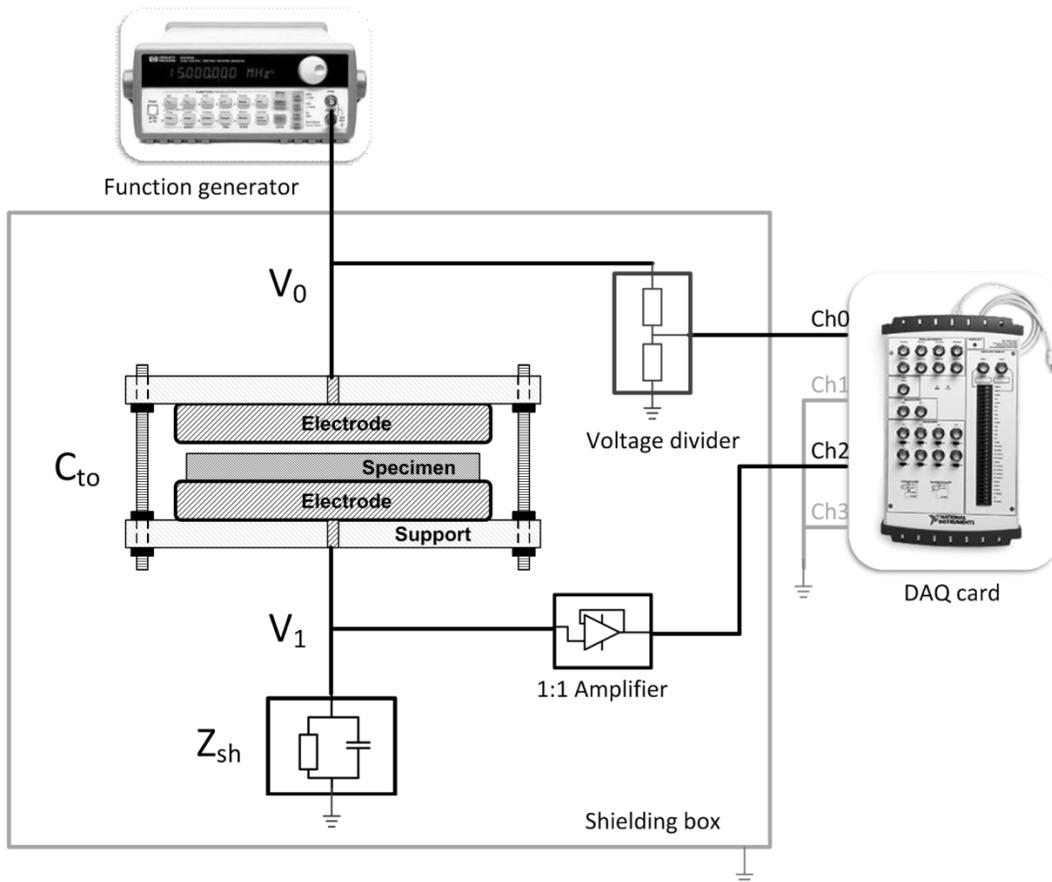
Figure 3.12: Schematic diagram of the experimental setup.
