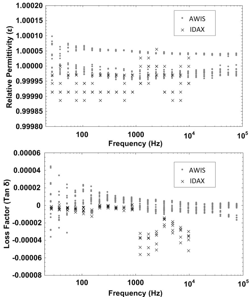
Figure 5.8: Relative permittivity and loss factor of air determined by air reference method with 3 different gap distances. These results indicate that base errors due to electrical measurement noise and drift in permittivity measurements are  $\pm 0.01\%$  and in  $\tan \delta$  measurements  $\pm 0.005\%$  for both AWIS and IDAX instruments.
