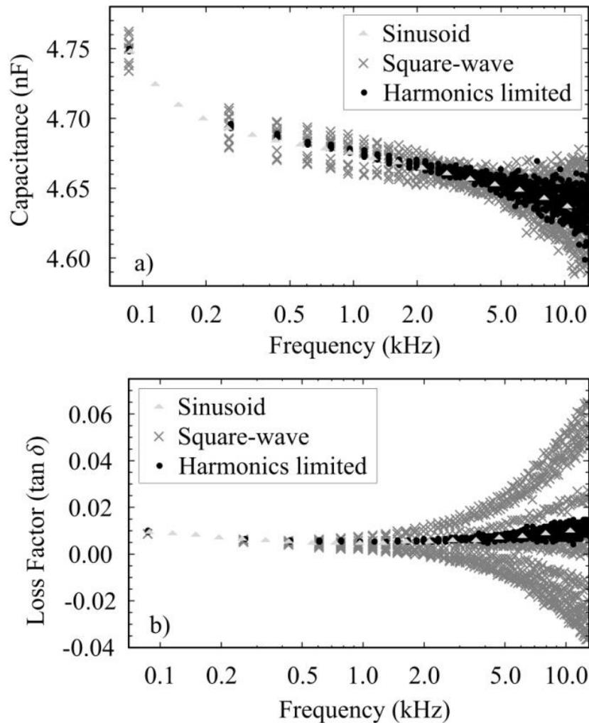
Figure 4.4: Comparison of ten individual measurements, a) capacitance and b) loss factor, obtained under a harmonics limited waveform ( $f_f = 80$  Hz, 10331 samples in the waveform, 75 odd harmonics) and under a square-wave waveform ( $f_f = 80$  Hz). As reference, a result obtained from swept measurement under sinusoidal waveform is shown.
