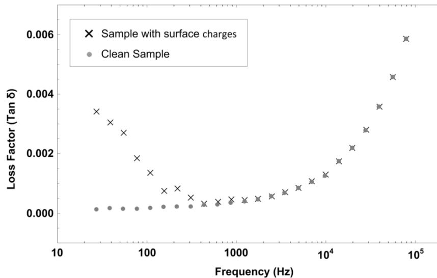
Figure 5.5: Results of two measurements of losses of a polycarbonate specimen with the same test gap using air reference method in contact-free electrode arrangement. In the first measurement, specimen was rubbed against hair to charge the surface; in the second measurement, specimen was cleaned by flushing the surface with isopropanol.
