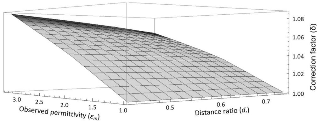
Figure 6.6: The plot of geometric correction factors ( $\delta$ ) for a 1 mm fixed test gap with respect to the observed permittivity ( $\epsilon_m$ ) and distance ratio ( $d_r$ ).
