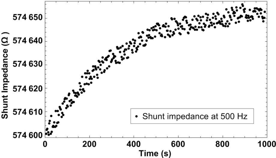
Figure 5.3: Measured impedance of current shunt at 500 Hz during 1000 seconds at constant current load. The noise level is visible by the distribution of individual measurement points
