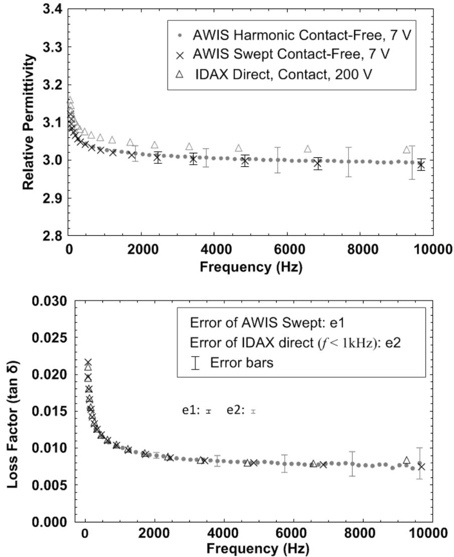
Figure 5.13: Relative permittivity ( $\epsilon_r$ ) and loss factor ( $\tan \delta$ ) of 1.92 mm thick EPDM rubber with ATH filler obtained by AWIS with contact-free electrode arrangement and air reference method with harmonic limited waveform (97.2 Hz fundamental frequency, 50 odd harmonics, 16000 samples in the waveform) and swept sinusoidal waveforms. As a reference, a result obtained by IDAX from swept sinusoidal waveforms and contact electrode arrangement is also shown.
