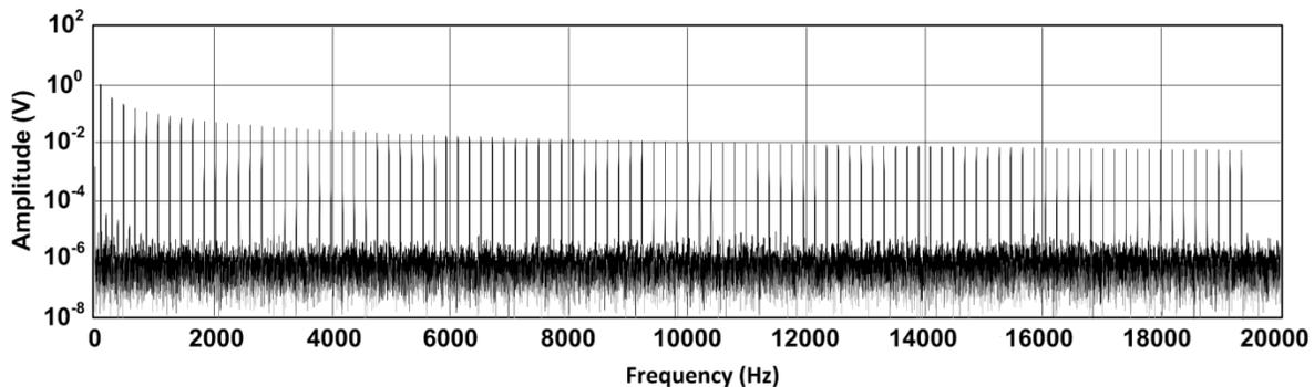
Figure 3.9: The measured voltage signal with a square like waveform which contains only 200 odd harmonics. The applied fundamental voltage is 1 V and 97.2 Hz. The sampling rate and measurement range are set to 200 kS/s and 2 V, and for each signal 270 kS are recorded for analysis.
