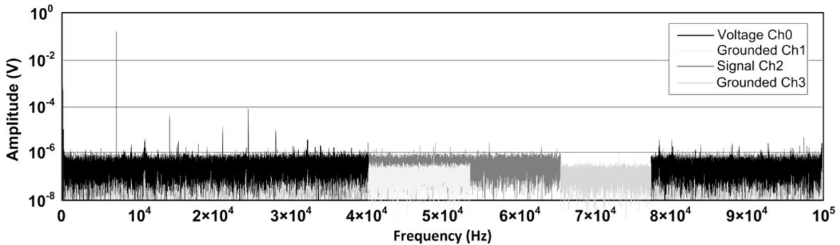
Figure 3.11: Noise levels of the whole frequency spectrum; a 1 V, 8 kHz sinusoidal voltage is measured through the voltage divider by Ch1 and its response signal over an air gap capacitor is measured by Ch2; responses of two grounded channels Ch1 and Ch2 are also shown. The sampling rate and measurement range of each channel is set to 200 kS/s and 1 V. For each signal, 270 kS are acquired and analyzed. In order to show the noise level of all signals, several parts are removed from the figure.
