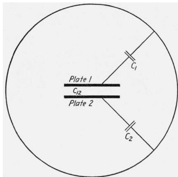
Figure 2.8: Diagram illustrating the coefficient of capacitance of two parallel plates with surroundings, copied from [3].
