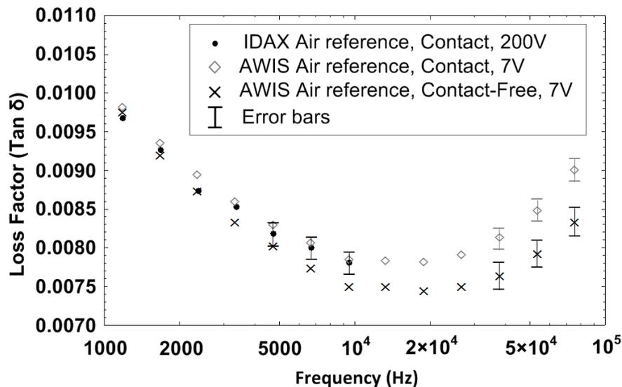
Figure 5.11: Loss factor of 1.93 mm thick EPDM with ATH filler specimen measured by AWIS and IDAX with different electrode arrangements, similarly to figure 5.9. In all the measurements, the air reference method was applied.
