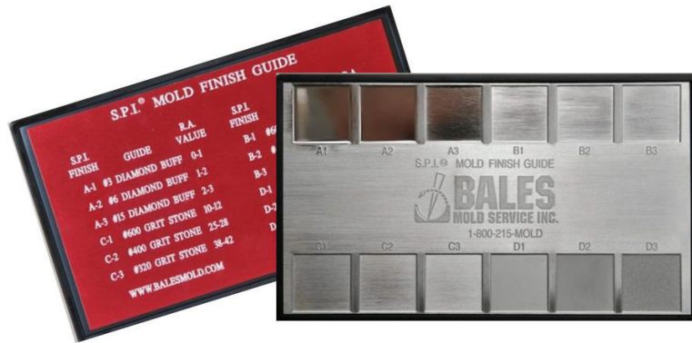
Figure 8: The Pocket S.P.I. Mold Finishing Guide providing short guidelines for surface preparation, expected surface finish and average roughness values.
