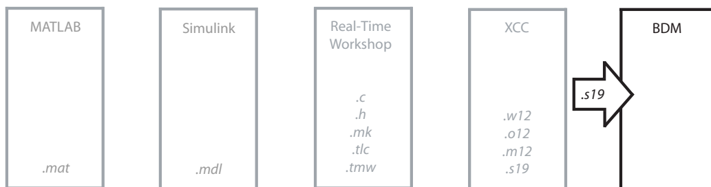
Figure 5.5 The compilation in XCC results in an executable .s19 file that via BDM is loaded on to the processor.
