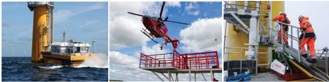
Figure 5-1: Example of transportation solutions for offshore wind farms. Left: Crew transfer vessel [76], middle: Helicopter hoisting [77], right: access system for Crew Transfer Vessel [78].
