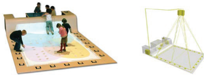
Figure 5.8. StorySurfer prototype installed at the library and a diagram of the set-up.
