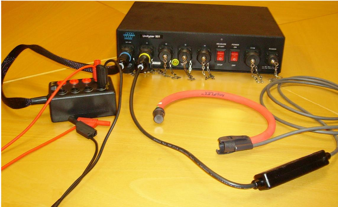
**Figure 11.** Measurement unit, Unilyzer 901. The small black box, seen to the left, is the coupling device for the voltage measurements and has four inputs. The orange coil, in the center, is a Rogowski coil used for AC current measurements.
