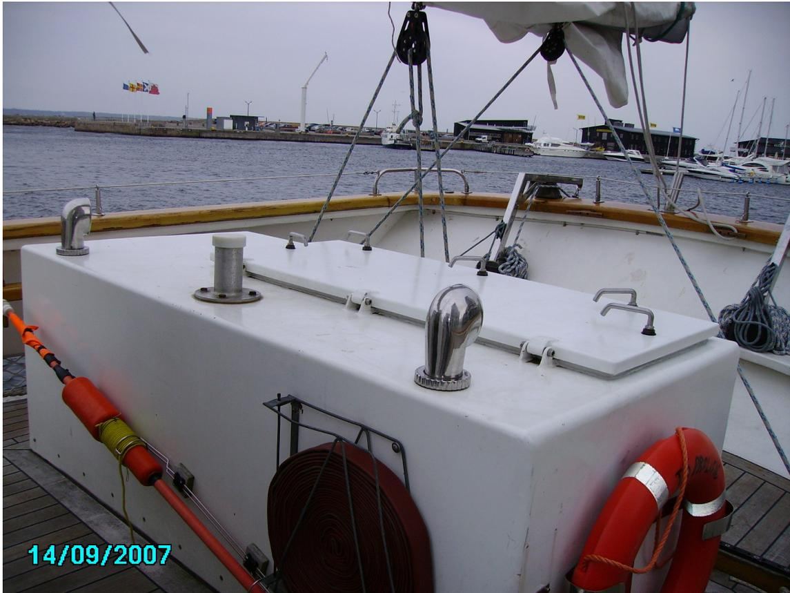
**Figure 24.** Over deck compartment for the possible placement of the fuel cell system.
