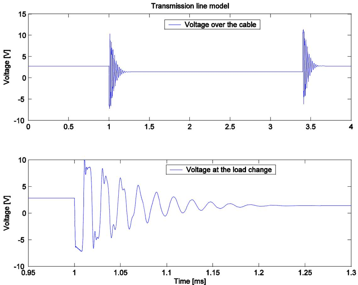
Figure 4.4 Transmission line model simulation, 1 – 2A pulsed current load
