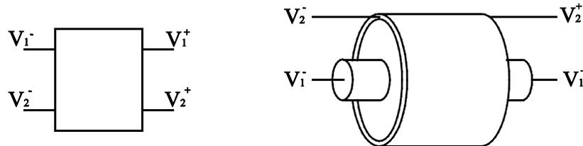
**Figure 2.12: A two port model, with reference directions and a corresponding coaxial cable with the S-parameter ports.**
