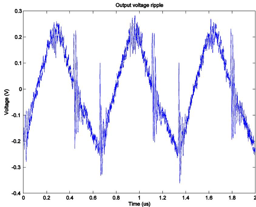
**Figure 5.6: Output voltage ripple at 3.5A load, full bandwidth**
