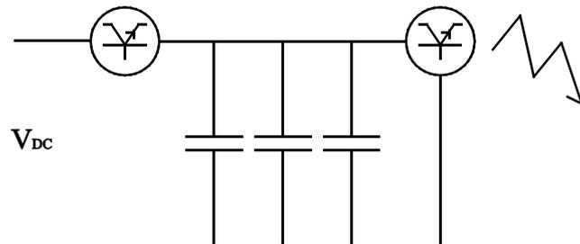
Figure 6.3 Approximate radar wave transmission circuit
