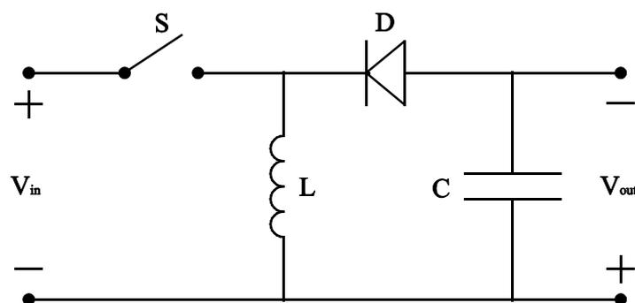
Figure 2.5 Buck boost converter topology
