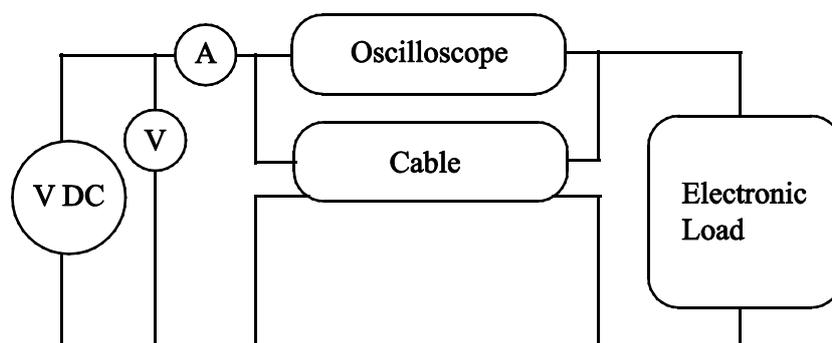
**Figure 4.6: The test setup for the coaxial cable measurement with the shield at both end connected to the minus pole of the DC power supply.**
