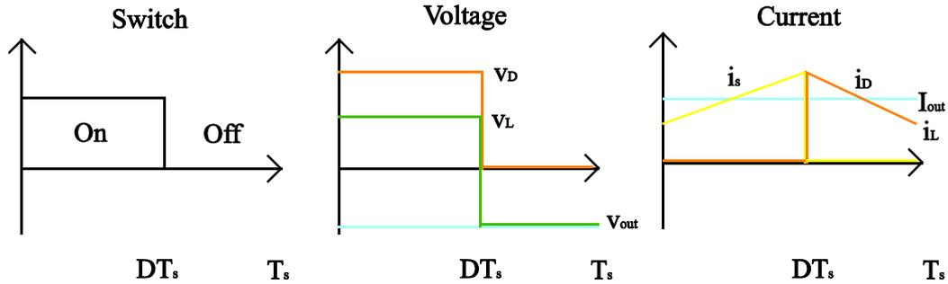
Figure 2.8 Switch, voltage and current waveforms in CCM over one switching period
