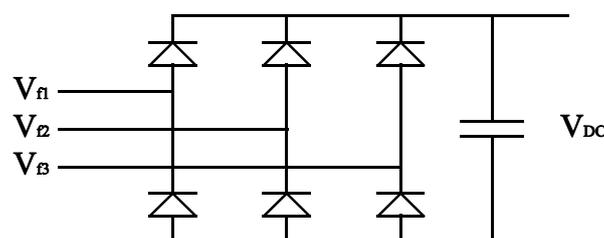
Figure 6.2 Full bridge rectifier with an output capacitor.
