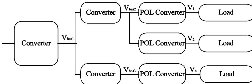
Figure 2.4 Intermediate bus architecture block diagram
