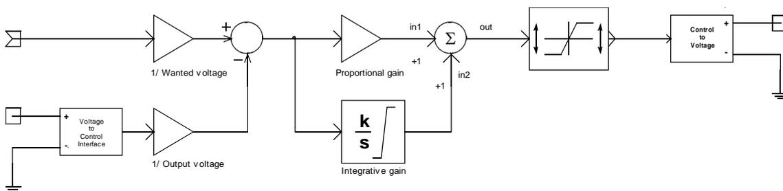
**Figure 5.3 PI regulated feedback design**
