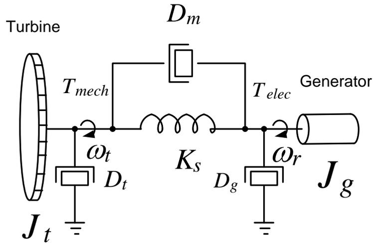
Figure 3.11: Drive Train of Wind Turbine
