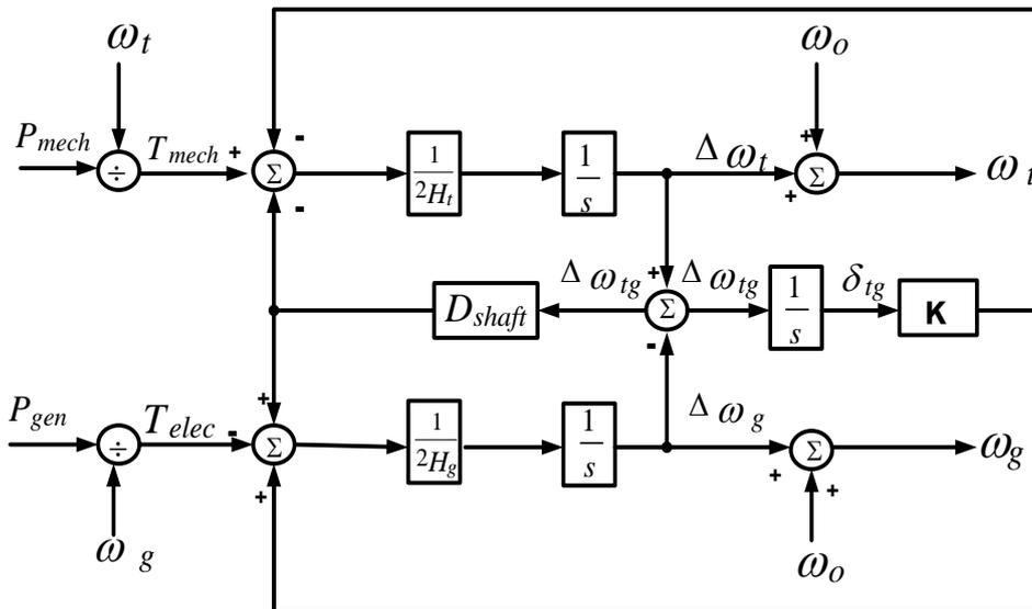
Figure 3.12: Two-mass torsional model
