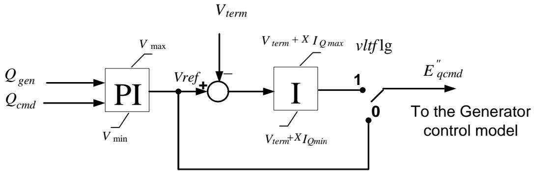
Figure 3.20: Voltage control model
