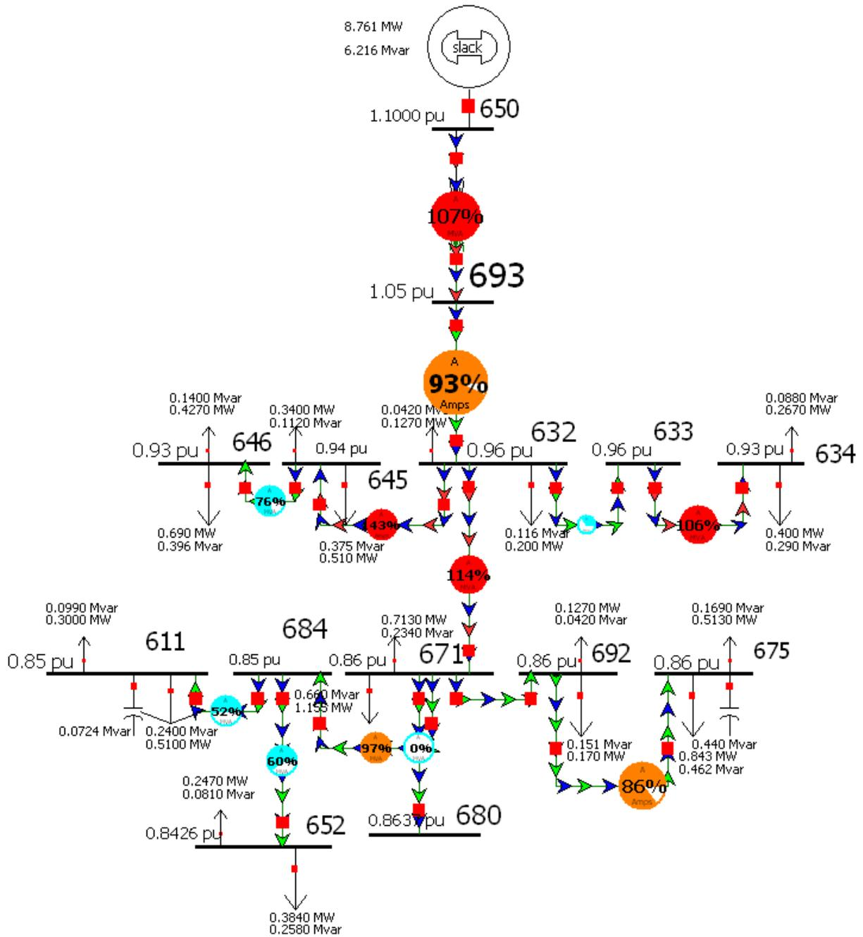
Figure 4: IEEE 13-node distribution test system with quick charging at peak load.
