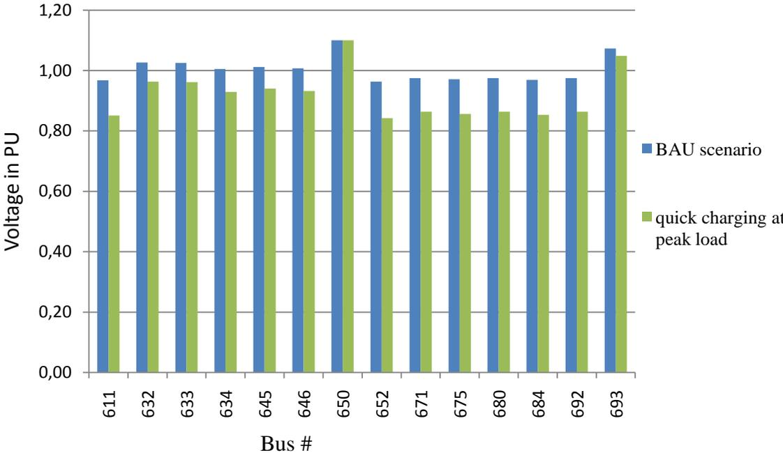
Figure 5: Bus voltages in BAU and quick charging at peak load
