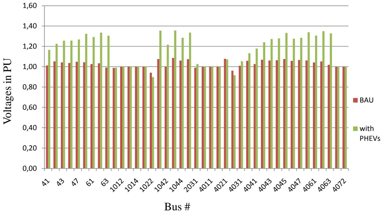
Figure 26: Voltage profile of the system before and after introduction of 10% penetration of the PHEVs
