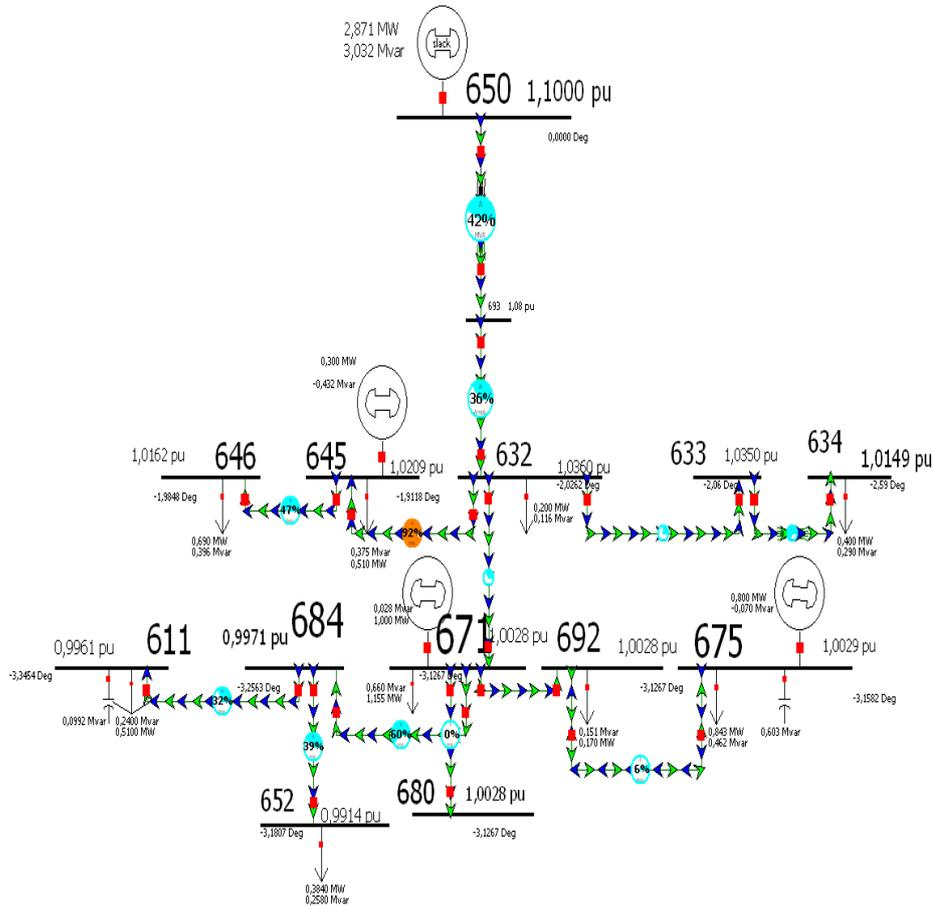
Figure 28: Over view of the IEEE 13- Node test system with some modification.
