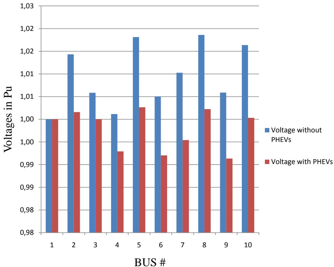
Figure 23: Different busses voltage with and without PHEVs
