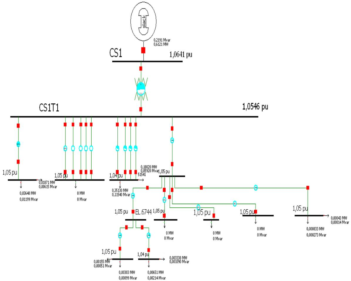
Figure 14: Single line diagram of commercial 400 V network connected to transformer 1 at substation CS1.
