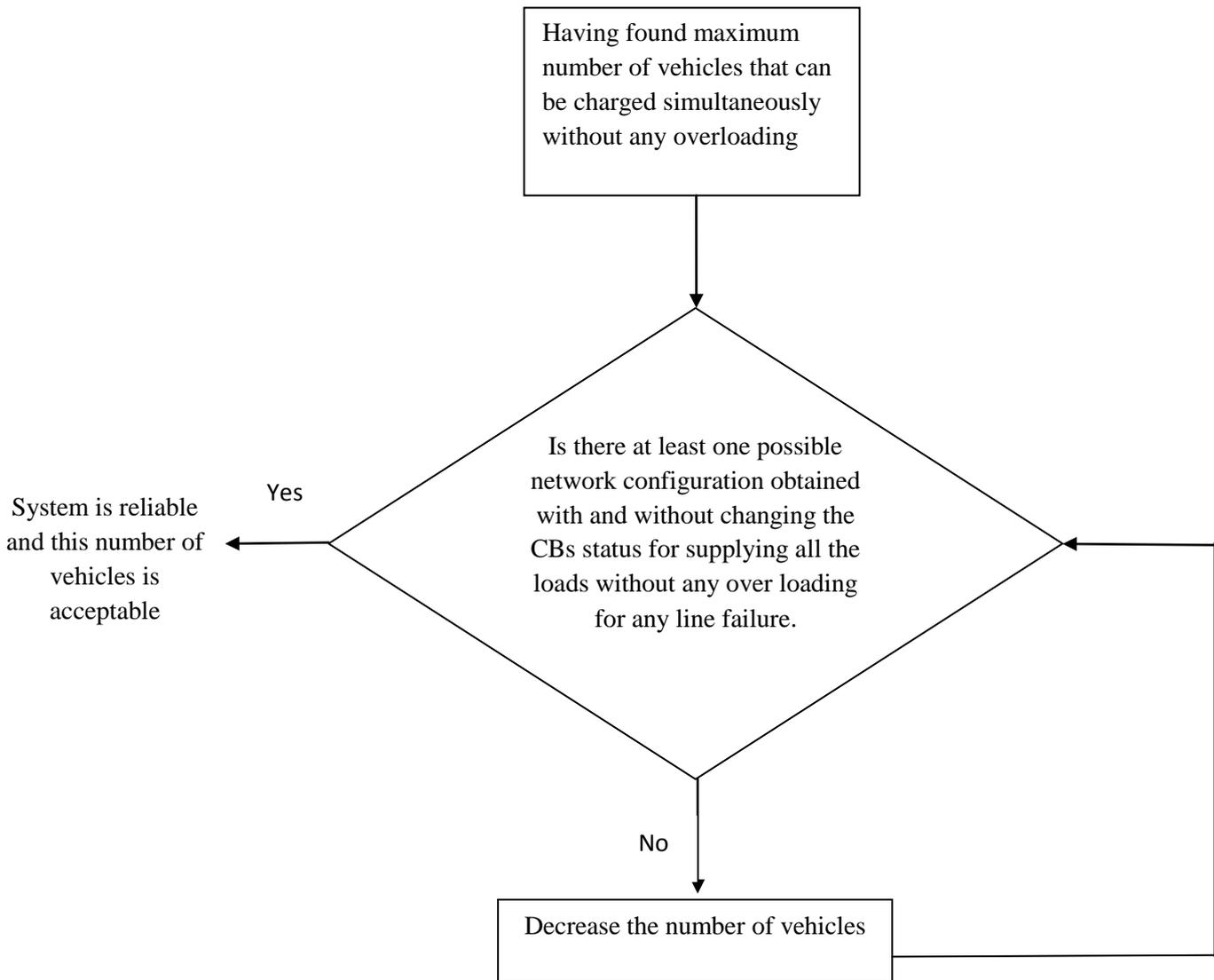
Figure 21: flow chart for checking the system reliability
