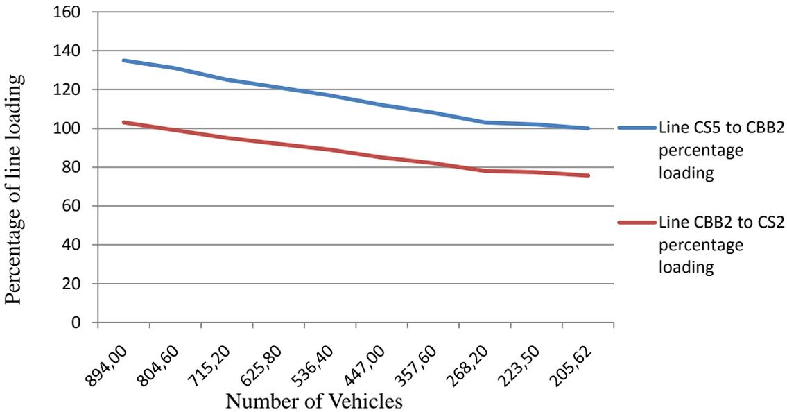
Figure 19: Percentage loading of 2 most loaded line in the commercial area versus different number of charging vehicles
