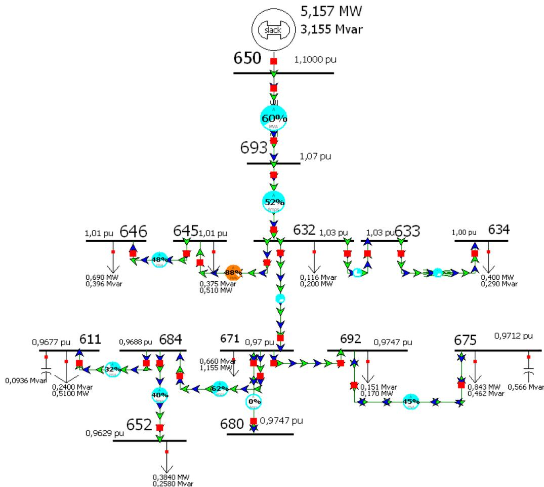
Figure 2: IEEE 13-Node test system without PHEVs.
