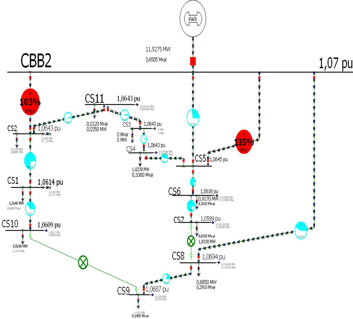
Figure 16: single line diagram of 10 kV network of the commercial area in Gothenburg.
