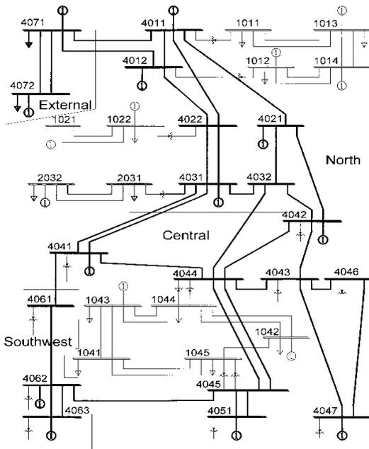
Fig. 4: Single line diagram of Nordic 32-bus system
