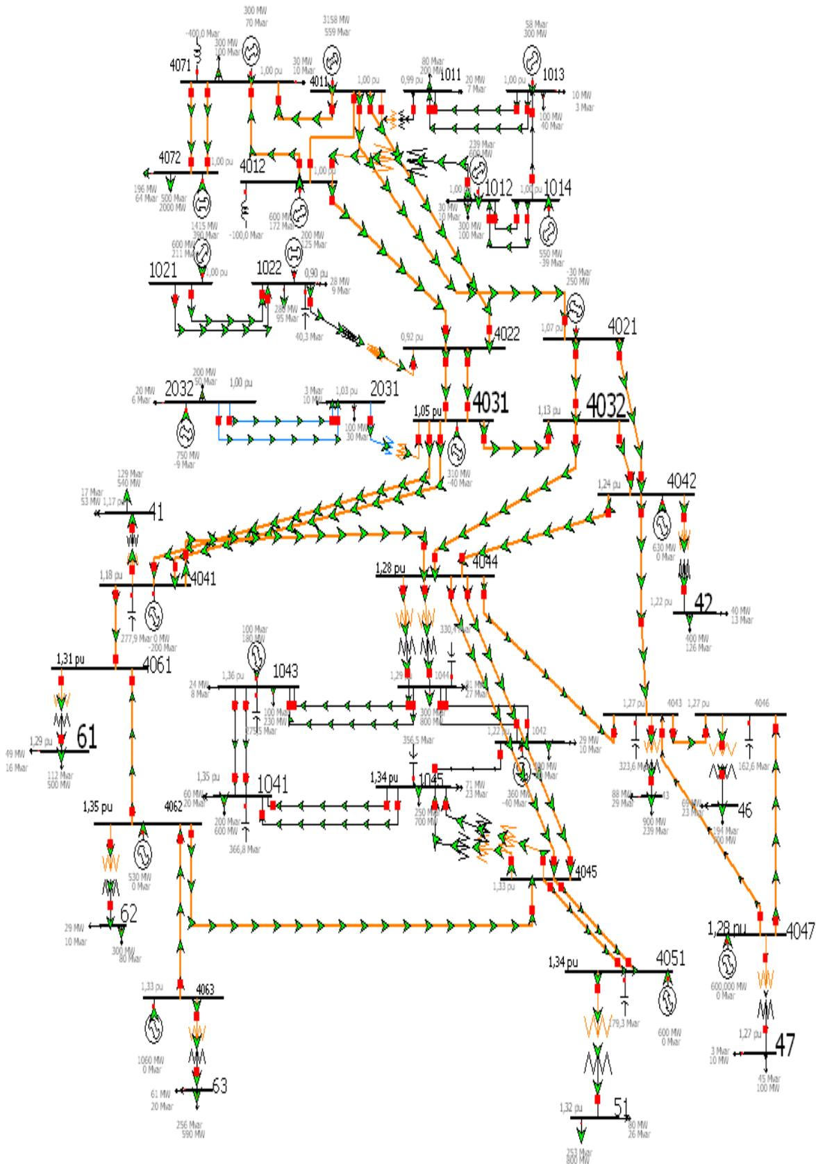
Figure 25: Nordic 32-Bus system with 10% penetration of PHEVs
