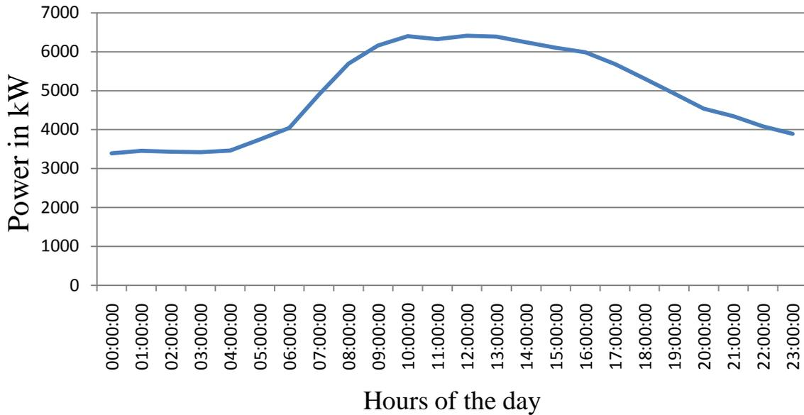
Figure 11: load profile of the 10 kV network supplying a commercial area in the Gothenburg on 14 February 2008.
