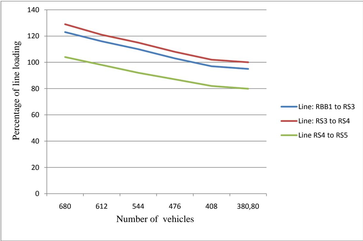
Figure 20: Percentage loading of 3 most loaded line in the residential area versus different number of charging vehicles
