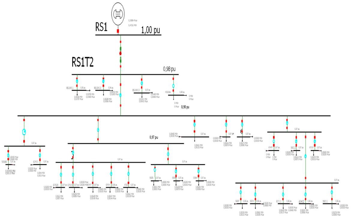
Figure 10: residential 400 V network connected to transformer 2 at substation RS1 while busbar RBB1 voltage is set at 1pu.
