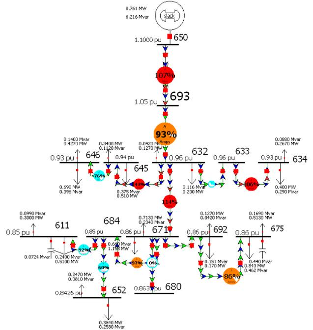
Fig. 2: IEEE 13-node distribution test system
