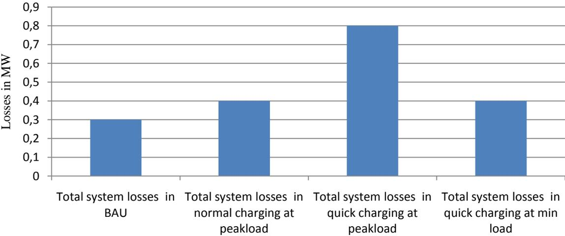
Figure 6: Total system active power losses
