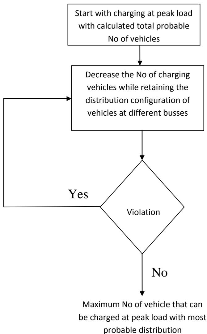
Figure 18: flow chart for calculation maximum possible charging
