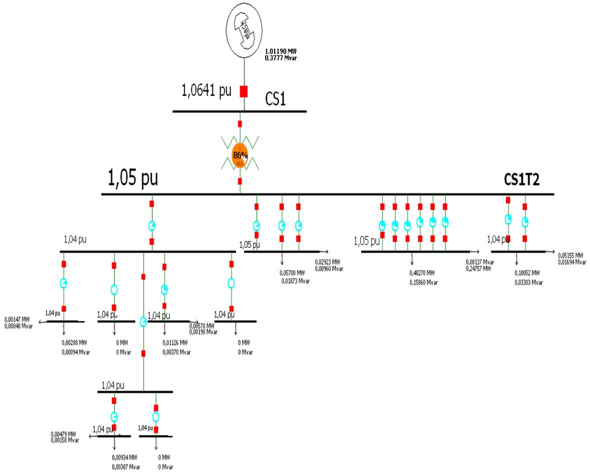
Figure 15: Single line diagram of commercial 400 V network connected to transformer 2 at substation CS1.
