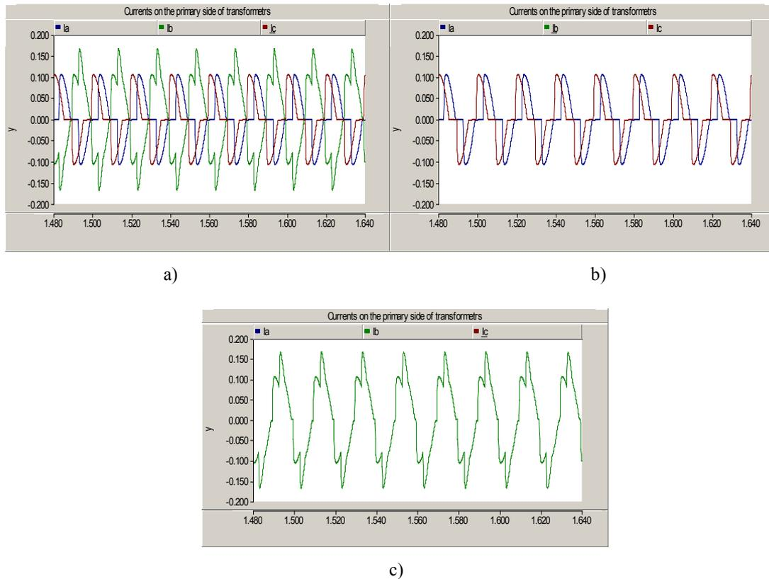
Figure (29): The currents on the primary side of transformers before filtering
