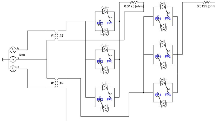
Figure 28. Schematic view of heating elements group furnace 6
