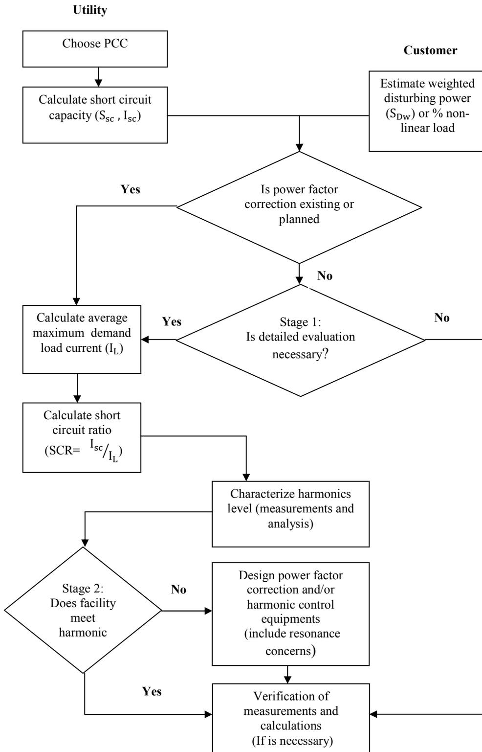
Figure 11. Process of harmonic evaluation
