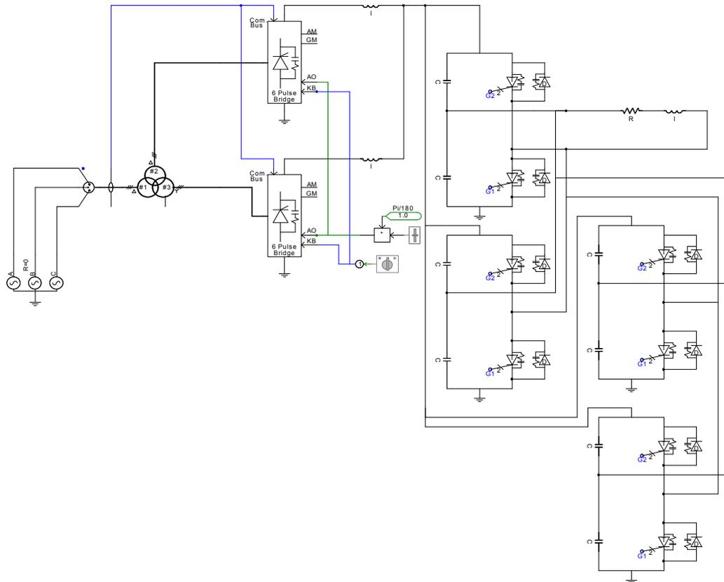
Figure 9. Simulated model of an induction furnace
