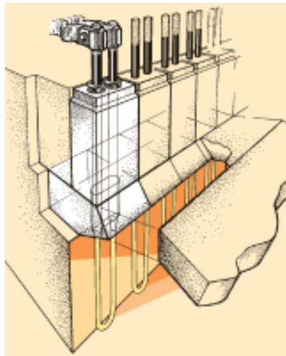
Figure 21. Installation of Sandvik Super elements with standard package bricks in a brick lined furnace
