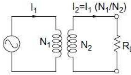
Figure 1 . Equal circuit of transformer
