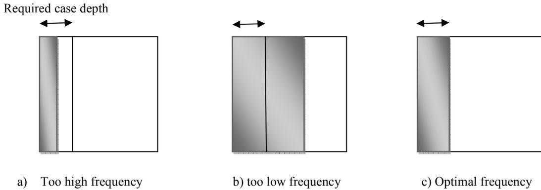
Figure 3. Current penetration depth
