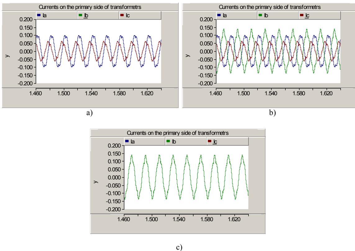
Figure (31): The currents on the primary side of transformers after filtering
