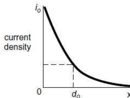
Figure 2 . Skin thickness and current density diagram
