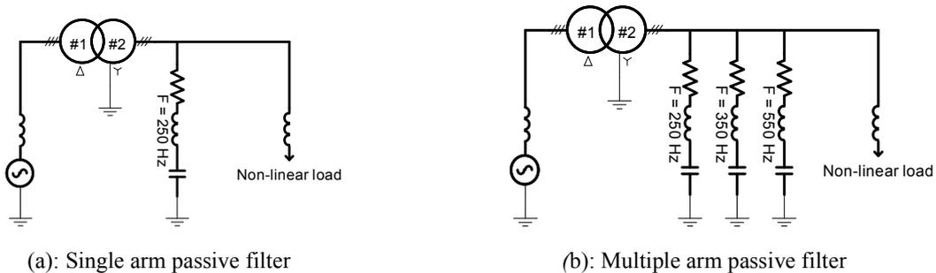
Figure 13. Passive filters
