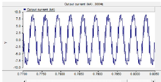
Figure 17. Output current to the work coil by 300Hz frequency
