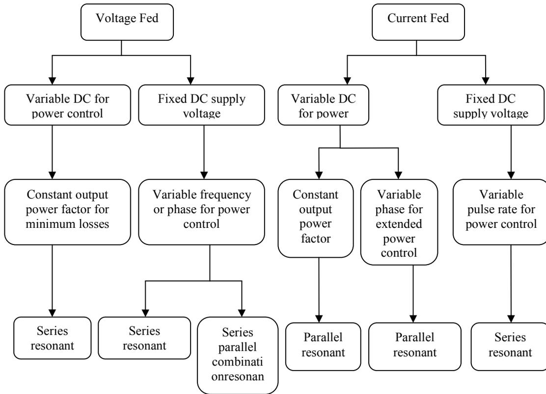
Figure 6. Induction heat inverters
