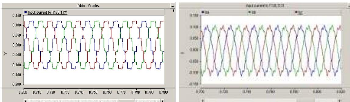
Figure 20. The currents on the primary side of T130 and T131 before filtering (left), and after filtering (right)
