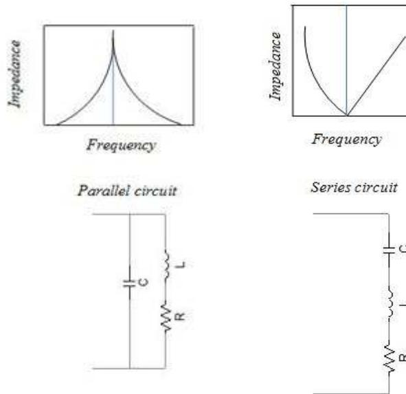
a) Parallel resonant                      b) Series resonant
