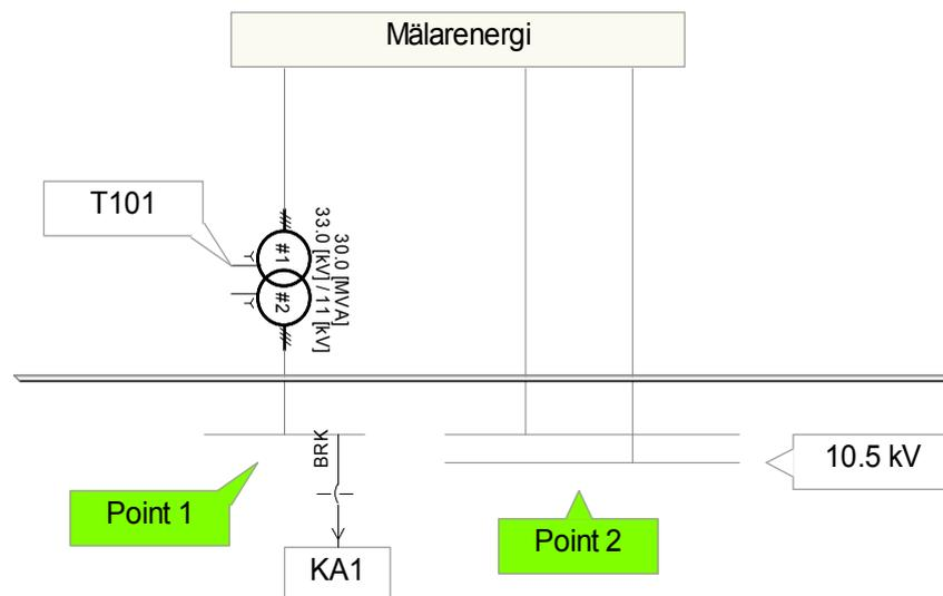
Figure 34. Overview of incoming electricity power to headquarter Company from Mälarenergi
