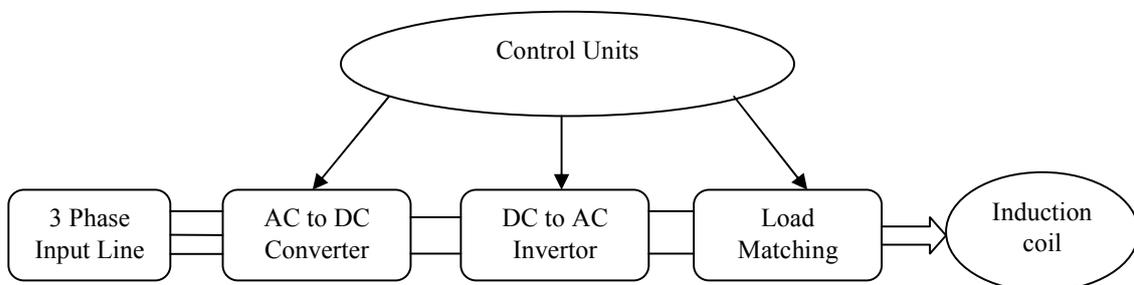
Figure 4. Basic block diagram of induction furnaces
