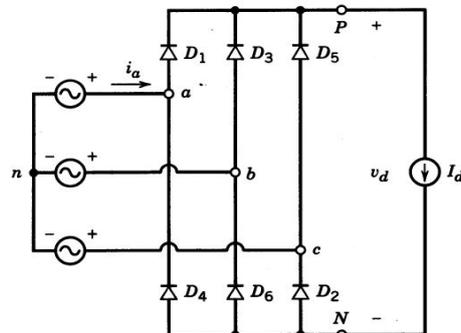
Figure 5. Full bridge converter
