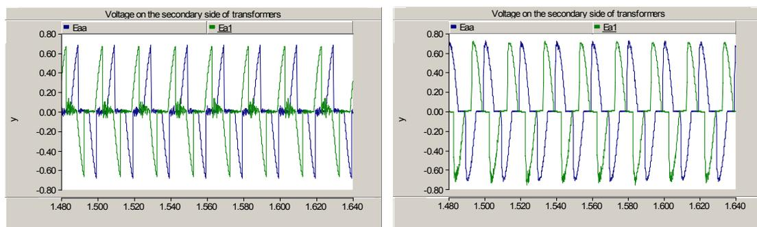
Figure 30. The voltages on the secondary side of transformers
