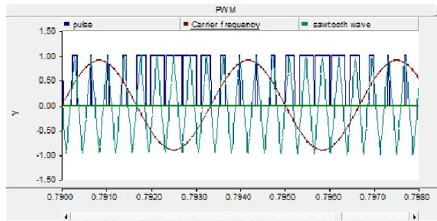
Figure 16. PWM control (ma=0.9 and mf=9)
