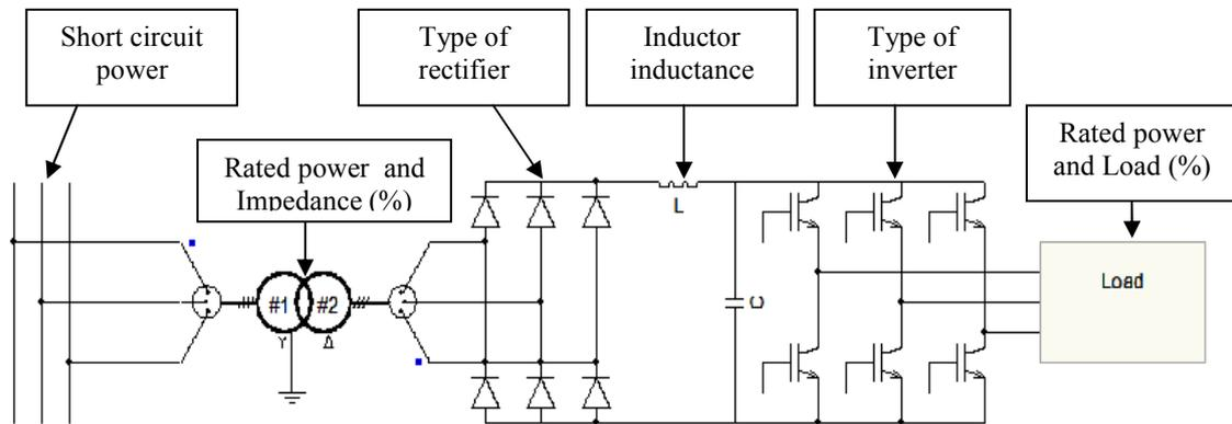
Figure 12. Drive system and affected harmonic factors
