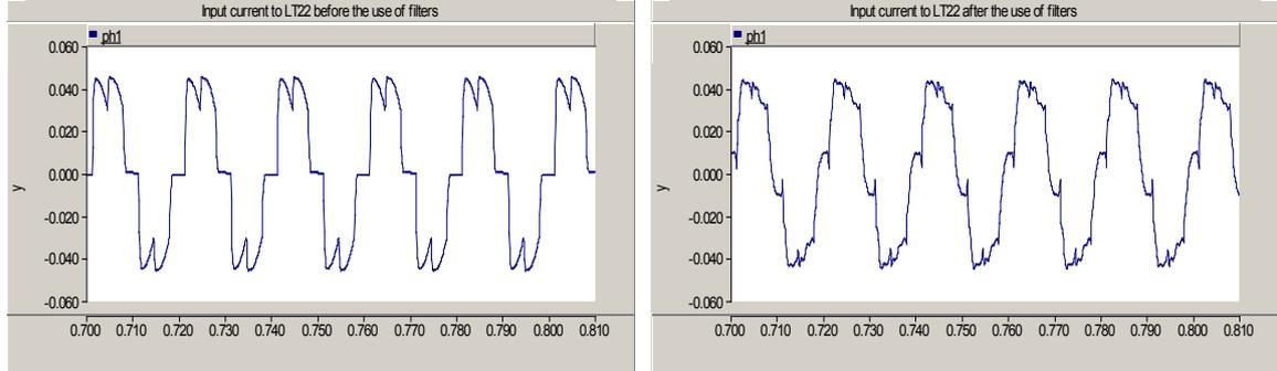
Figure 27. Single phase view of current on the primary side of LT22 before filtering (left), and after filtering (right)
