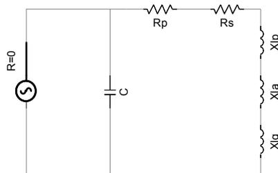
Figure 8. Equivalent circuit for an induction heating load
