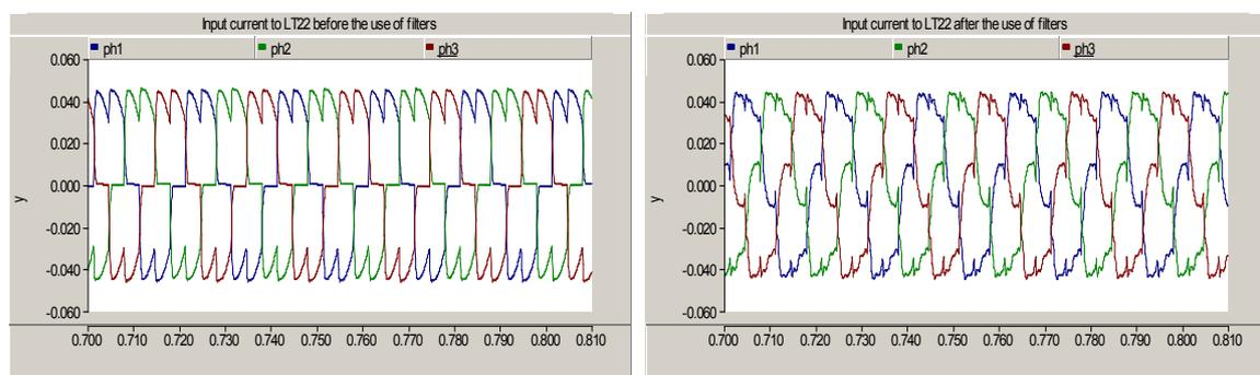
Figure 26. The currents on the primary side of LT22 before filtering (left), and after filtering (right)
