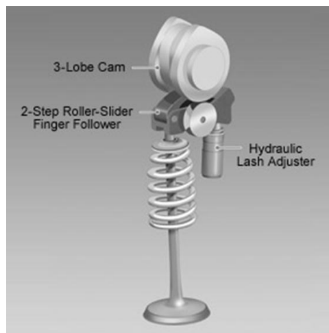
Figure 10: Delphi switching finger follower [19]
