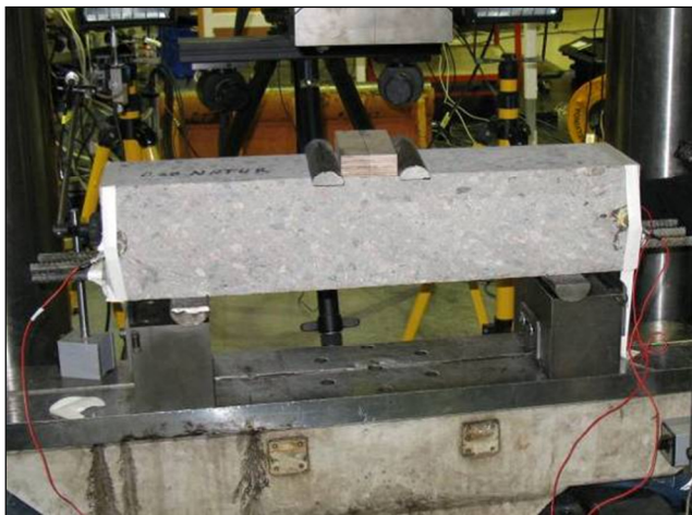
Figure 3.3 The shear test set-up of the RC beams with the optical measuring system showing in the background and the placing of the AE-sensors at each end of the beam.
