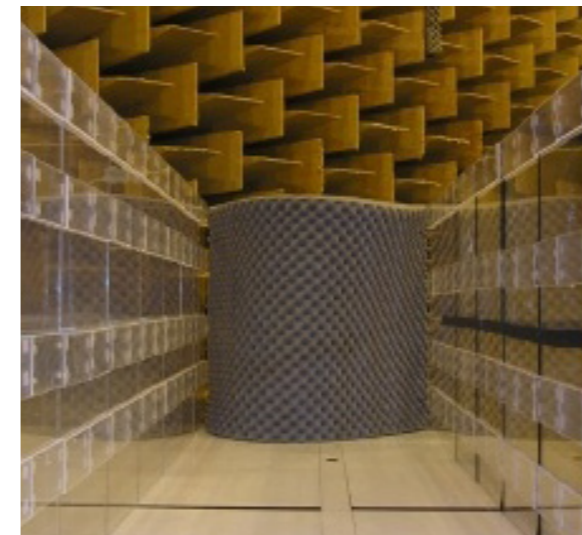
Figure 4. A scale model of a city canyon (a street with high buildings on both sides) for experimental investigation of sound propagation in urban environments.
