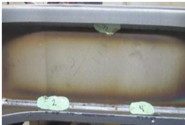
Fig. 5 Polymer applied to weld to get impressions.
