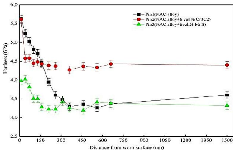
Fig.2 Nano-hardness versus surface distance in the subsurface layer of pin 1#, pin 2# and pin 3#.
