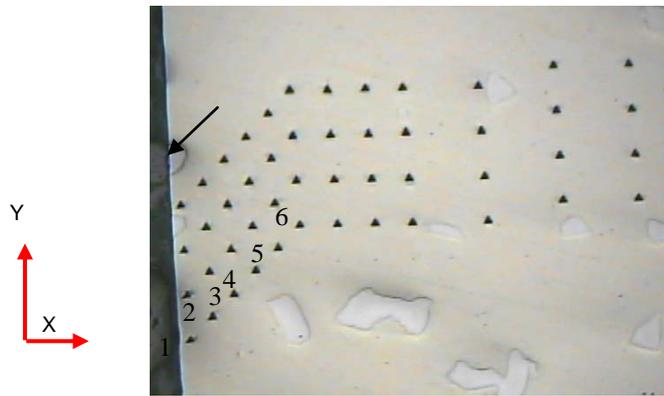
Fig.1 A map of the indents in the subsurface layer of pin 2#. An arrow indicated the worn surface.
