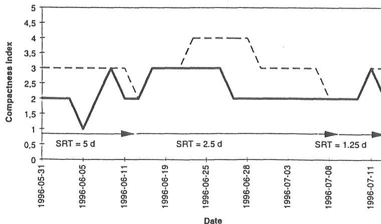
Figure 4 b. Compactness index, part III (dotted line=A; continuous line=B; A: 0.5 mg O<sub>2</sub>/l; B: 2.0 mg O<sub>2</sub>/l).
