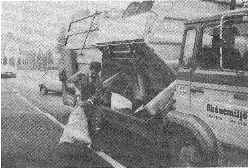
Figure 6.5 The Squirrel. A four-chamber vehicle constructed for the N rab Recycling System.
