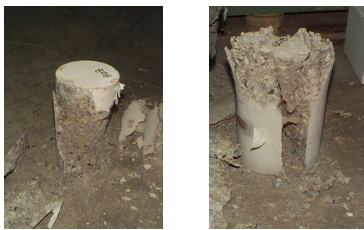
Figure 3. Cylinder failures, left with friction and right with Teflon layers removing friction.
