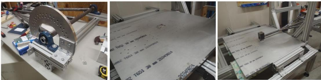
*Appendix F 4 a) Assembled bearing solution, charge angle plate and hammer arm
