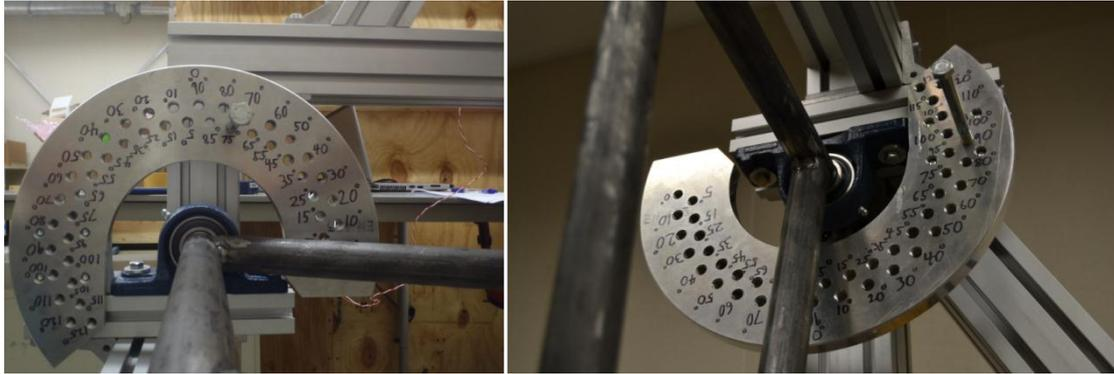
Figure 79 Charge angle plate in a) OOP configuration b) IP configuration
