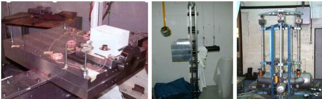
Figure 10 Example of metal-to-metal impact STFs a) mono-plate b) bi-plate c) tunable plate [16]
