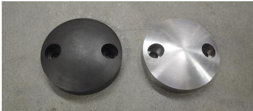
*Figure 87* The two different hammerheads. The hammerhead on the left is the hardened one
