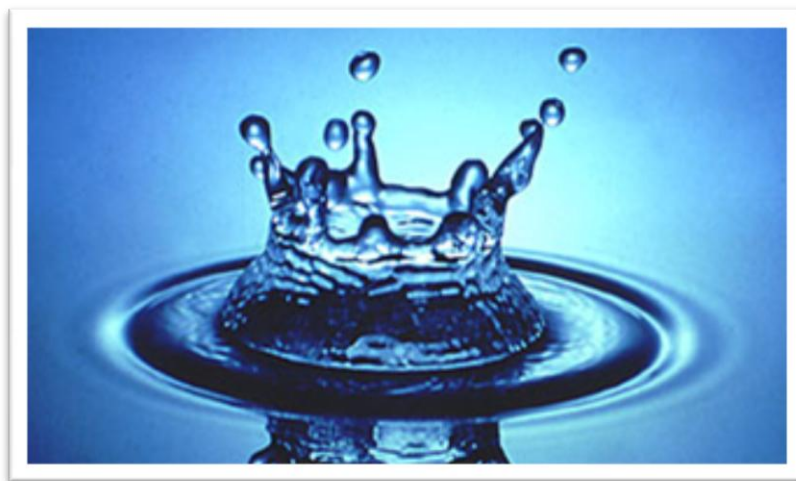
Fig. 13. Impacting water droplet crown formation. Secondary droplets can be seen leaving the crown rim.
