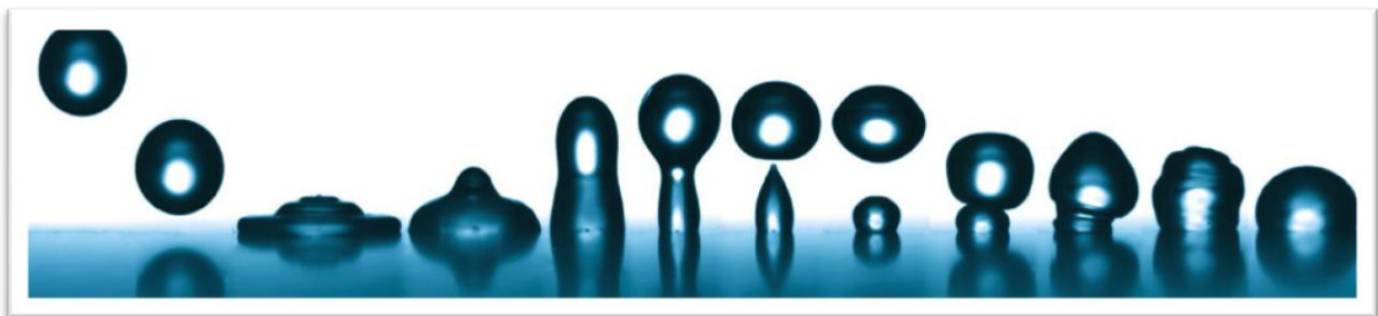
Fig. 12. Droplet impacting and partly rebounding from a dry rigid wall (ME Department, 2012).
