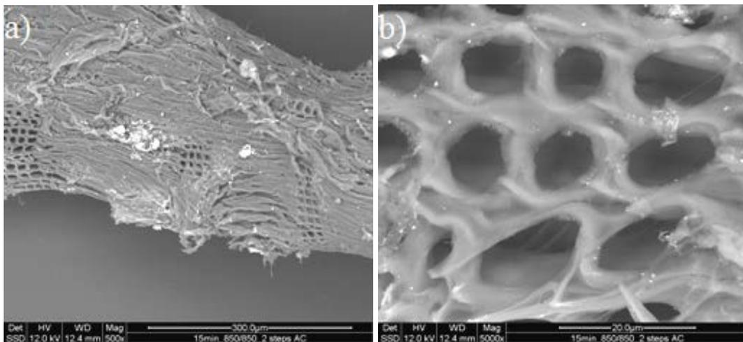
Figure 5.16: SEM images of the activated carbon produced by two steps method at T=850°C, t=15min and LSF a) mag.500X, b) mag.5000X
