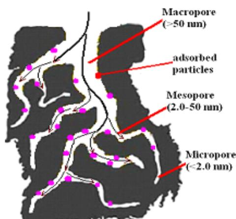
Figure 3.2: Schematic picture of the pores inside the activated carbon (figure created by C. Charles) [12]
