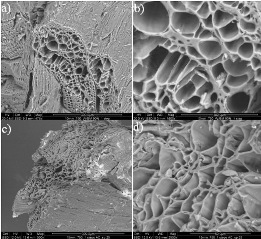
Figure 5.13: SEM images of the activated carbon, produced by one step method at 750°C, a)  $t=10\text{min}$ , HSF, (mag. 476X), b)  $t=10\text{min}$ , HSF (mag. 1600X), c)  $t=15\text{min}$ , LSF (mag. 500X), d)  $t=15\text{min}$ , LSF mag. 2500X)
