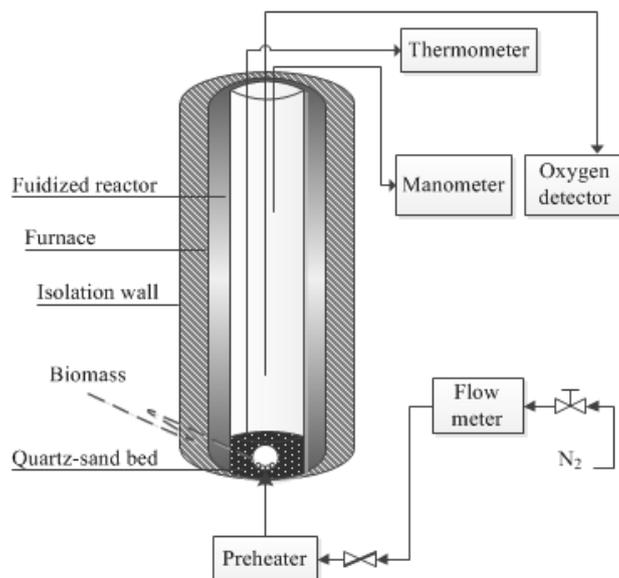
Figure 4.1: Schematic diagram of the vertical fluidized bed reactor set-up
