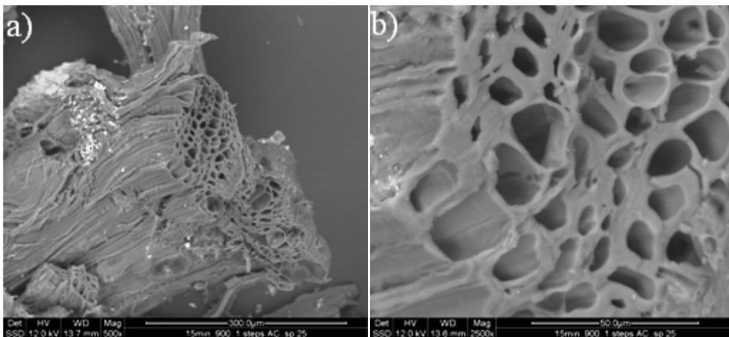
Figure 5.18: SEM images of the activated carbon produced by one step method at  $T=900^{\circ}\text{C}$ ,  $t=15\text{min}$  and LSF a) (mag.500X), b) (mag.2500X)
