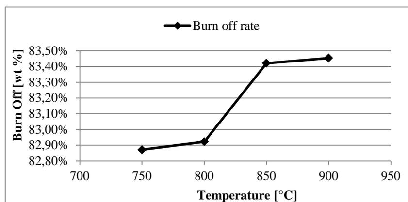
Figure 5.1: Burn off vs. temperature during the pyrolysis of wood pellets.  $t=5$ min ( $\sigma = 0.22\%-0.54\%$ , standard deviations for five samples at each temperature)
