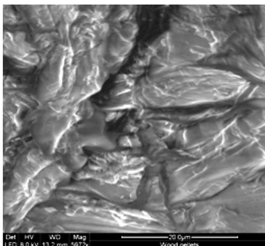
*Figure 5.11: SEM image of a virgin wood pellet used in the experiments (mag.5000X)*
