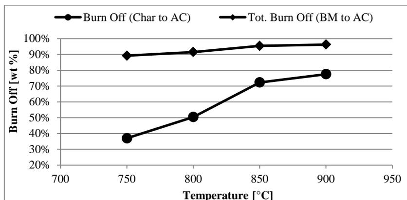
Figure 5.2: Variation of the burn off and total burn off with temperature during the production of activated carbon by the two-steps activation method.  $t=15\text{ min}$ , LSF
