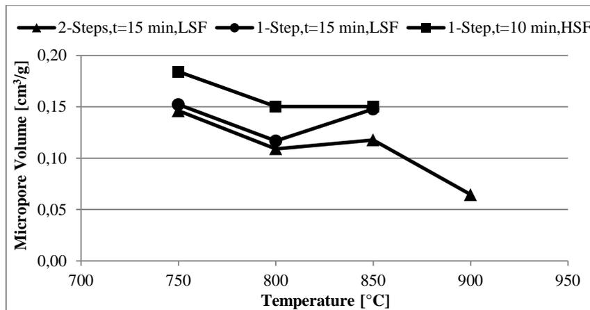
Figure 5.10: Effect of the operating temperature on the development of the total micropore volume of the samples of AC produced by 1 and 2-steps methods
