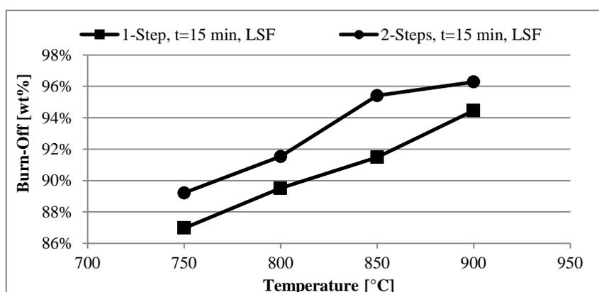
Figure 5.6: The effect of temperature on the total burn off for the samples of activated carbons produced by 1 and 2-steps activation methods. t=15 min, LSF
