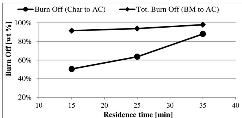
Figure 5.3: Variation of the burn off and total burn off with residence time during the production of activated carbon by the two-step activation method  $T=800°C$ , LSF
