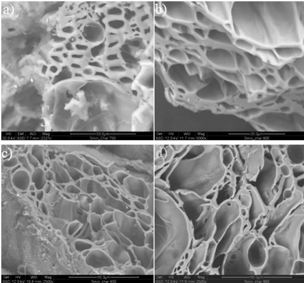
*Figure 5.12: SEM images of the char samples produced during pyrolysis at 5 minutes residence time and operating temperatures of a) 750°C (mag. 2327X), b) 800°C (mag. 5000X), c) 850°C (mag.2500X), and d) 900°C (mag. 2500X)*
