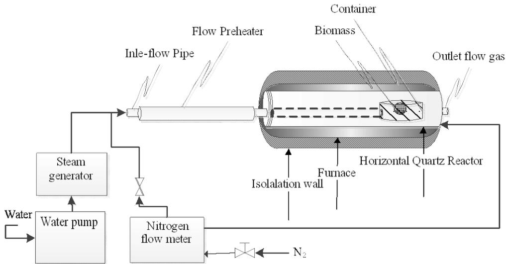
Figure 4.2: Schematic diagram of the horizontal quartz reactor set up
