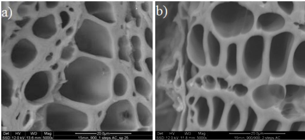
Figure 5.17: SEM images of activated carbon produced at 900°C and, t=15 min and LSF a) one step method b) two-steps (mag.5000X)
