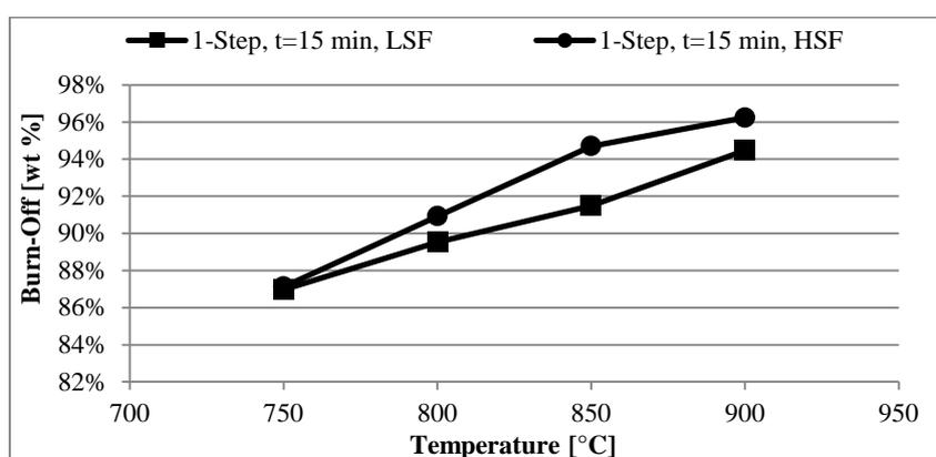
Figure 5.5: Variation of burn off with steam flow 1-step, t=15 min
