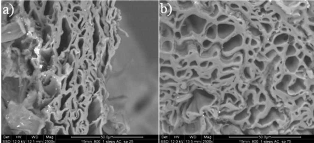
Figure 5.15: SEM images of the activated carbon produced by one step method at T=800°C and t=15min a) LSF (mag.2500X), b) HSF (mag.2500X)
