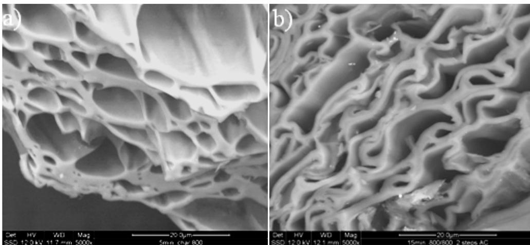
Figure 5.14: SEM images of char and activated carbon produced at  $T=800^\circ\text{C}$  a) char,  $t=5\text{min}$  (mag.5000X), b) AC, 2-steps method,  $t=15\text{ min}$ , LSF (mag. 5000X)
