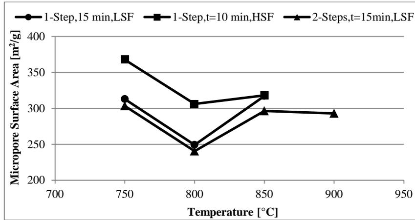
Figure 5.8: Effect of the operating temperature on the micropore surface area of the samples of AC produced by 1 and 2 steps methods
