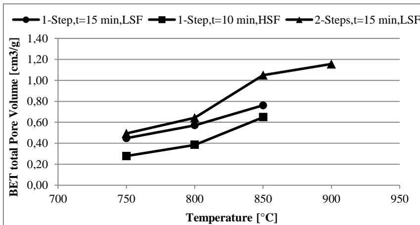
Figure 5.9: Effect of the operating temperature on the development of BET total pore volume of the samples of AC produced by 1 and 2-steps methods
