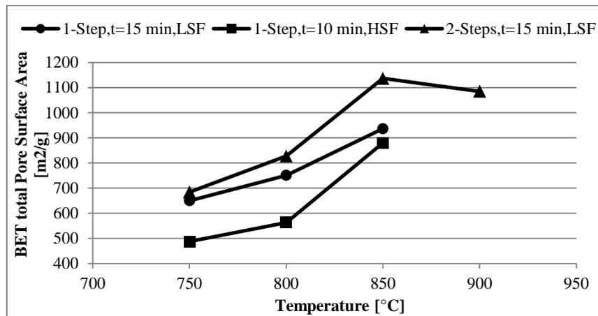
Figure 5.7: Effect of the operating temperature on the BET total pore surface area of the samples of AC produced by 1 and 2-steps methods
