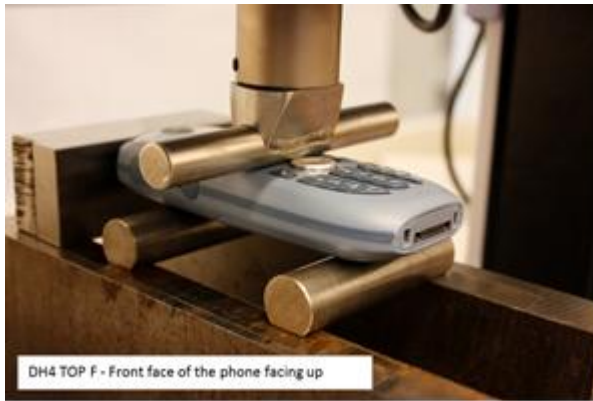
Figure 26 - Front side loading on DH4 handset
