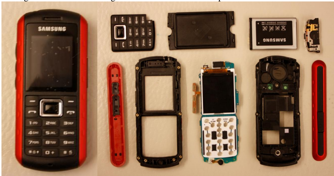
Figure 18 - Samsung X2100 disassembled parts
