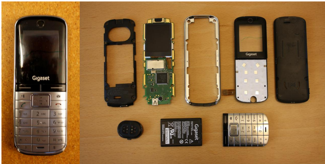
Figure 13 - Siemens SL400 disassembled parts
