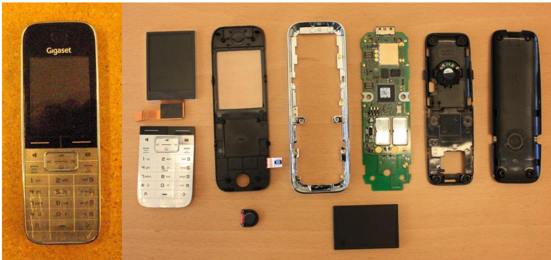
Figure 11 - Siemens SL78H disassembled parts
