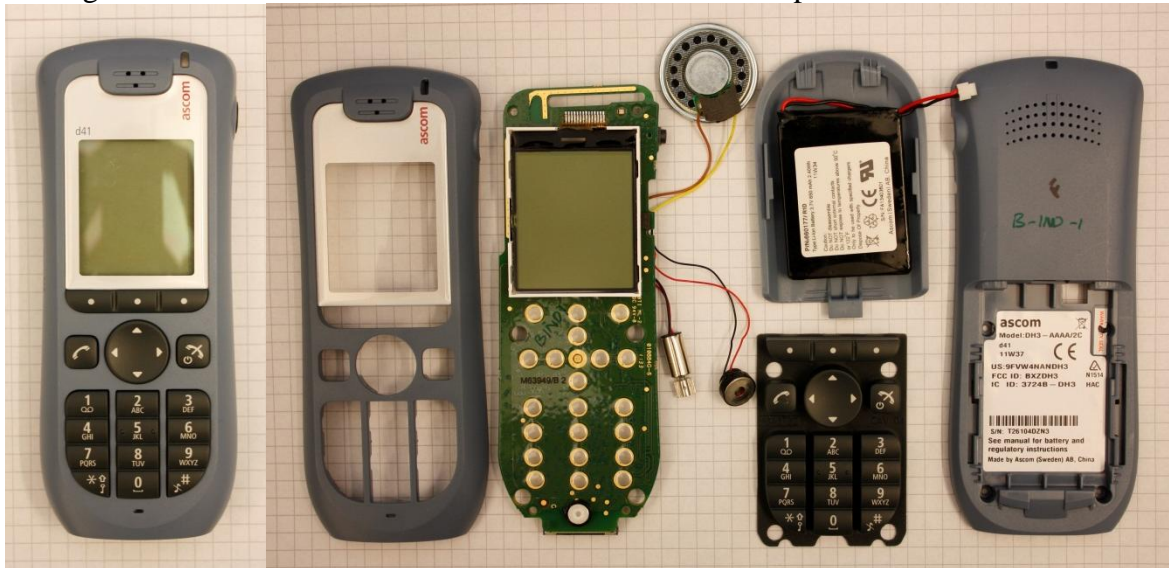
Figure 2 - DH3 handset disassembled parts
