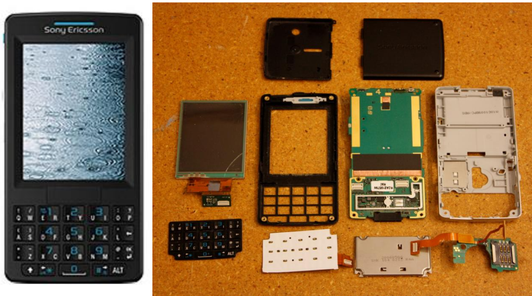
Figure 16 - Sony Ericsson M600i disassembled parts
