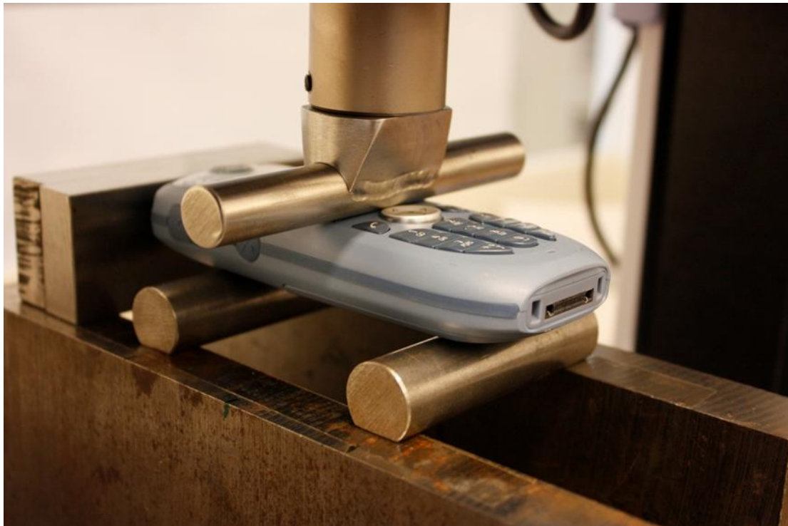
Figure 22 - DH4 tested with the Bending test probe
