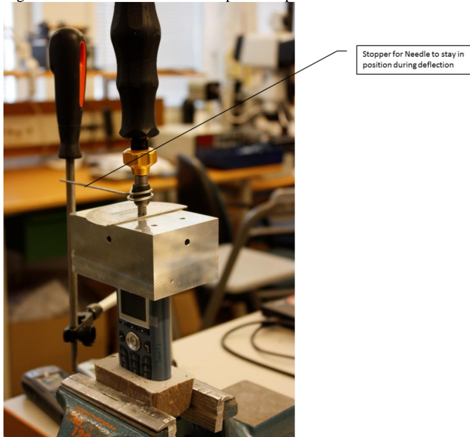
Figure 25 - Twist test set up in hold position
