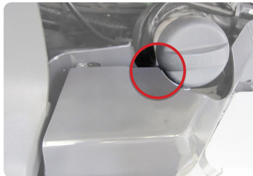
Figure 10-8 Washer fluid container clearance
