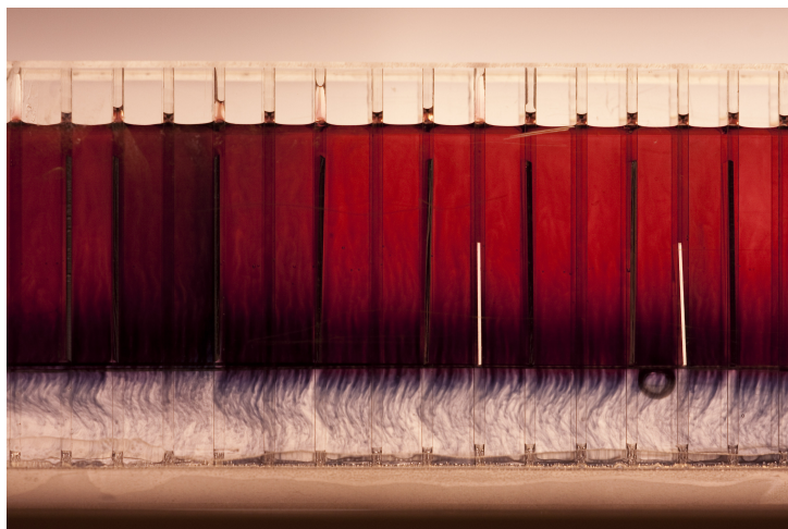
Figure 3.2: Photograph showing the simultaneous coating of multiple surfaces with gradients of Au NPs. Specifically, the brightly and darkly coloured vertically placed substrates correspond to gold coated glass and silicon substrates respectively. It is, moreover, possible to distinguish a bluish region between the upper nanoparticle suspension, which has a deep red colour, and the, relatively, clear concentrated buffer found at the bottom of the container. Specifically, this intermediate layer is formed due to the coagulation of the particulate matter, which in turn is a result of the high buffer concentration.
